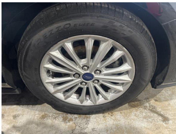
2: Wheel osf Scratched Over 50mm
