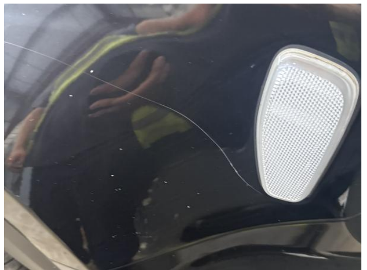
14: Wing osf Scratched Over 25mm Thru Paint
