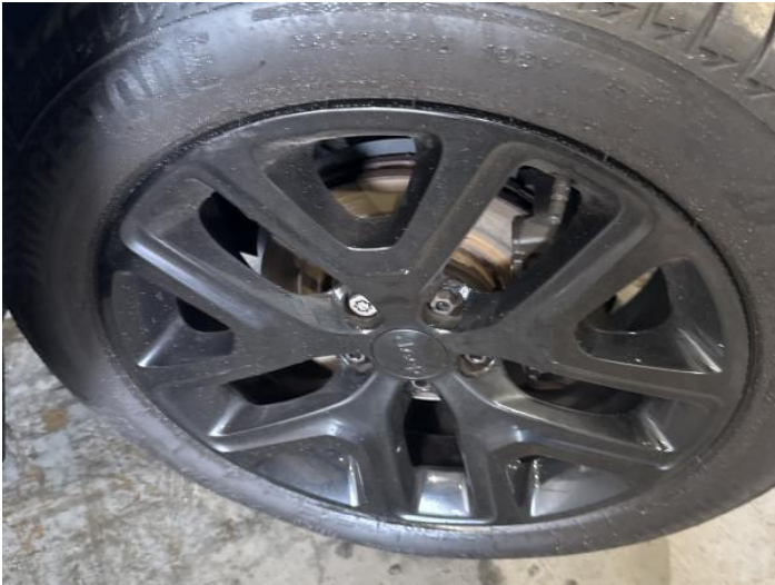
15: Wheel osf Scratched Up To 50mm
