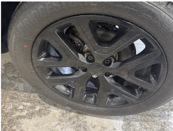
5: Wheel nsr Scratched Up To 50mm
