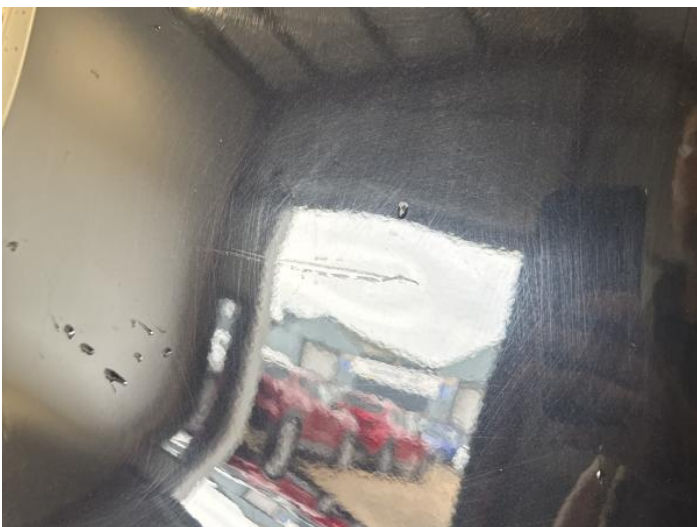
19: Qtr Panel osr Dented With Paint Damage
