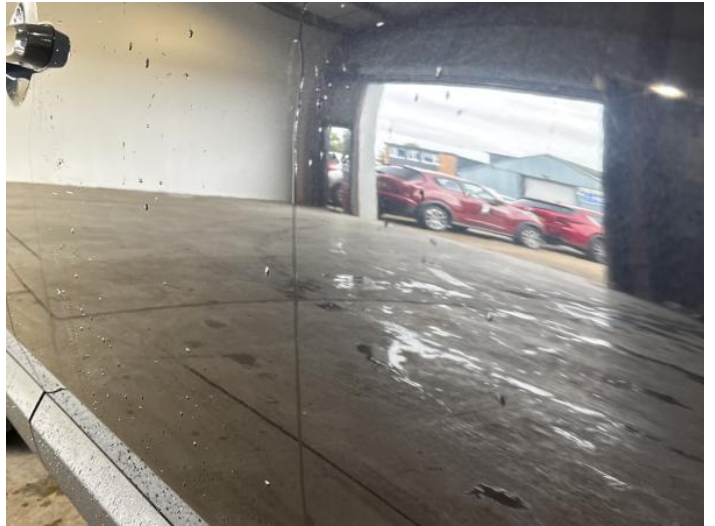
16: Door osf Dented 2 Or Less UpTo 10mm
