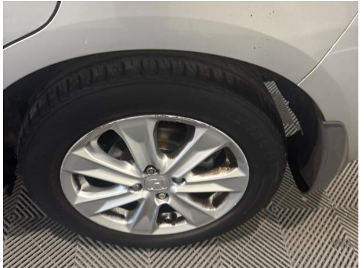
10: Wheel nsr Scratched Over 50mm
