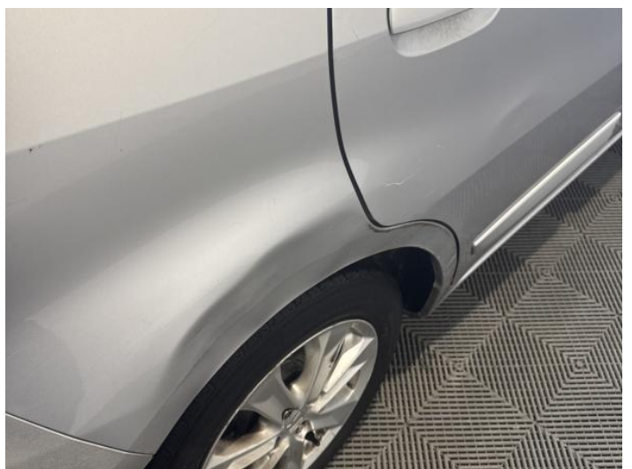
14: Qtr Panel osr Dented Over 30% Of Panel
