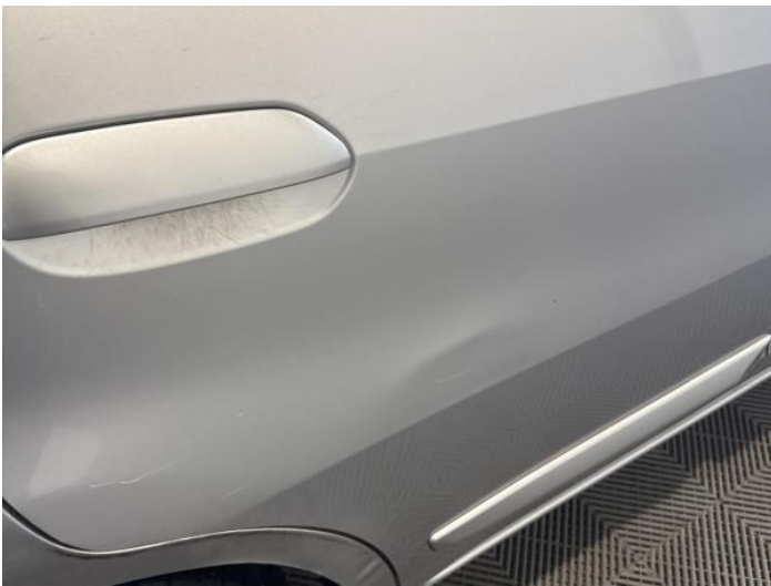
17: Door osr Dented With Paint Damage
