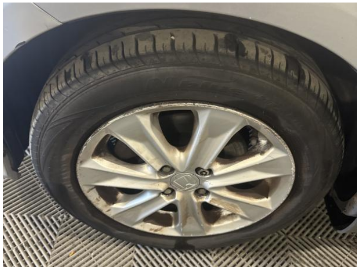
4: Wheel nsf Scratched Over 50mm
