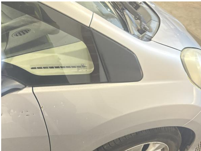
21: Wing osf Dented With Paint Damage
