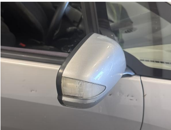
19: Door Mirror Assy osf Scratched (Painted) Over 25mm Thru Paint
