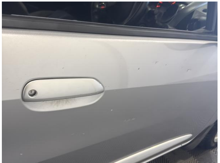
18: Door osf Dented With Paint Damage
