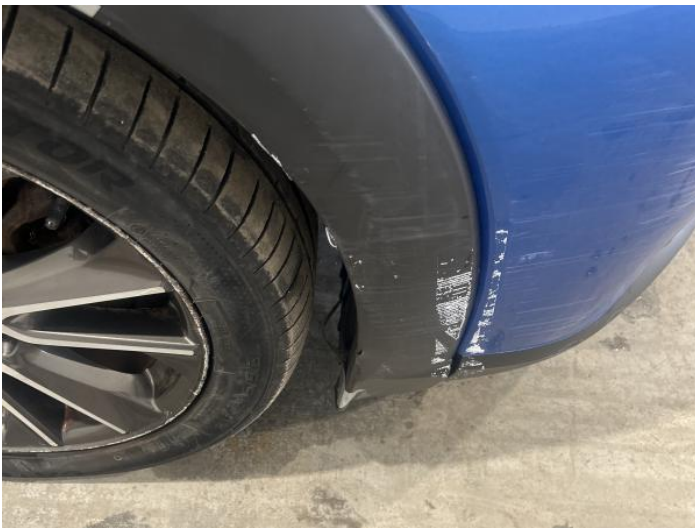
1: Qtr Panel Arch Extension os Scuffed (Unpainted) Over 100mm
