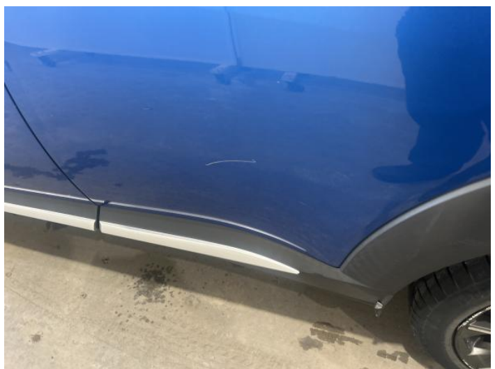
8: Door nsr Scratched Over 25mm Thru Paint
