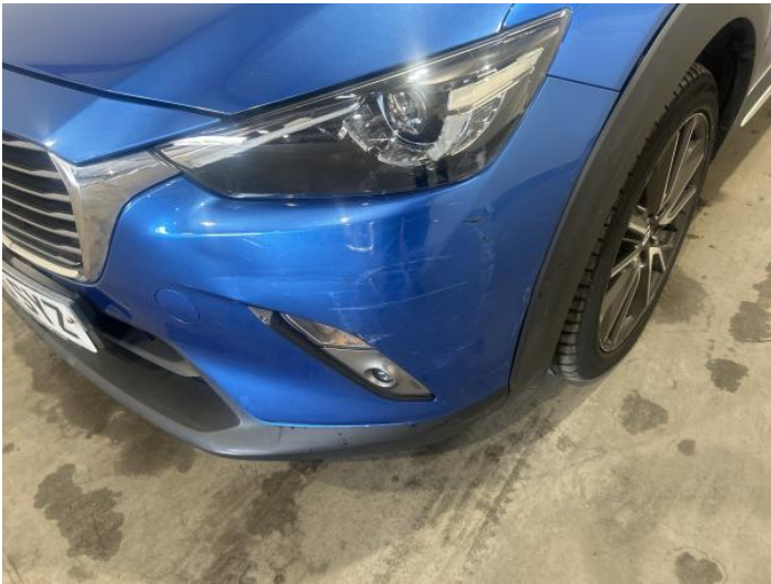
11: Bumper Front Scratched Over 100mm Thru Paint
