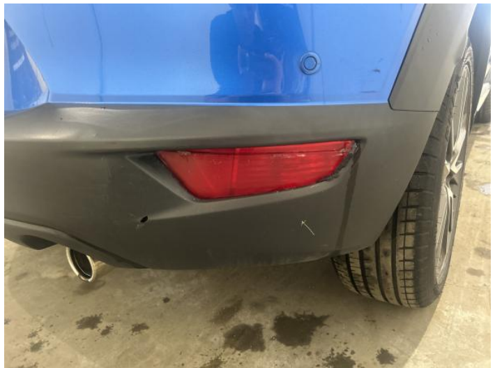
4: Reflector osr Broken Replace
