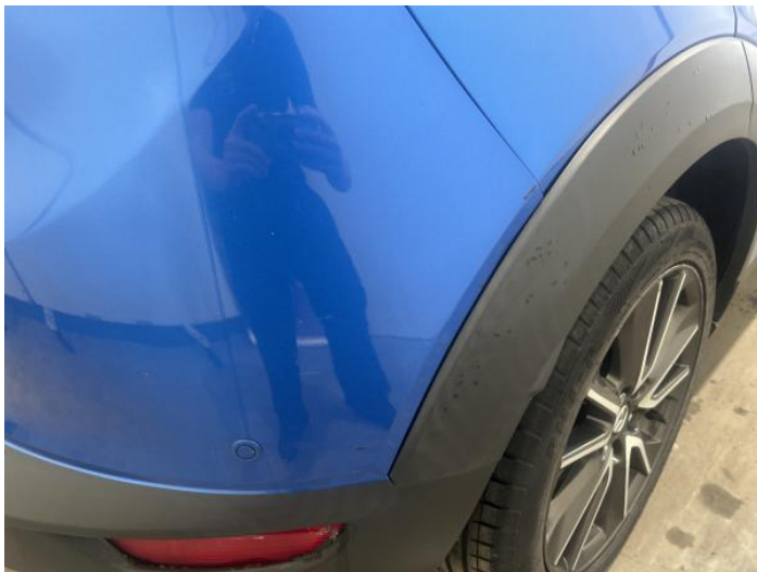
5: Bumper Rear Scratched 25 to 100mm Thru Paint
