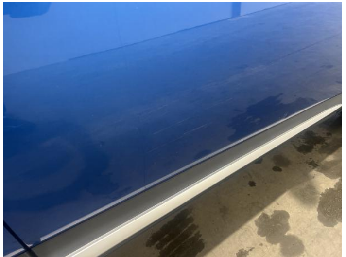
2: Door osf Scratched Over 25mm Thru Paint
