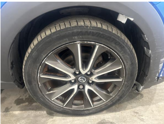
13: Wheel osf Scratched Over 50mm
