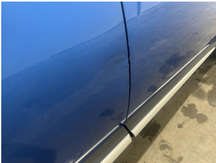
3: Door osr Dented Over 30mm
