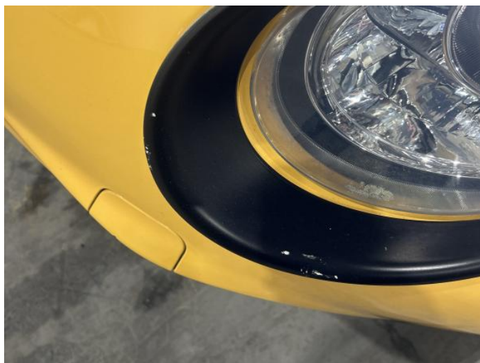
6: Fog Lamp Surround ns Scratched (Painted) Over 25mm Thru Paint
