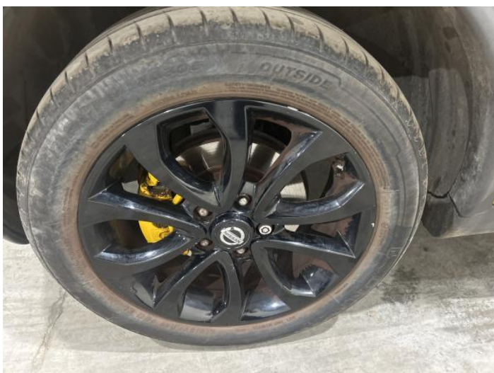
7: Wheel nsf Scratched Up To 50mm
