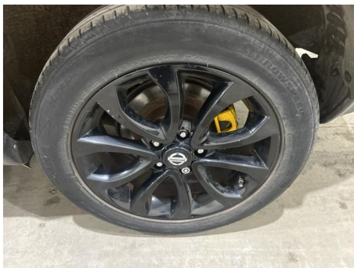
8: Wheel nsr Scratched Up To 50mm
