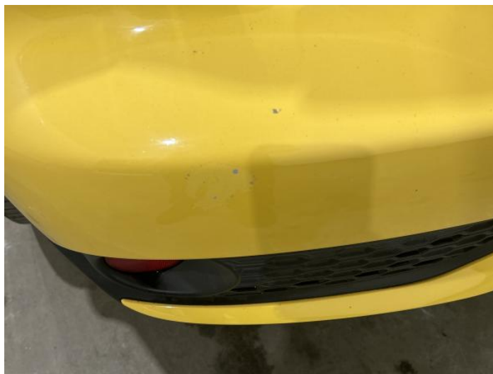
2: Bumper Rear Poor Previous Repair Paint Flake
