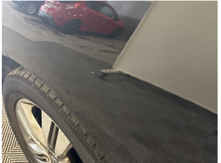
4: Wing nsf Scratched Over 25mm Thru Paint
