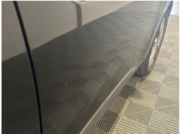
12: Door osf Poor Previous Repair Rippled UpTo 30%
