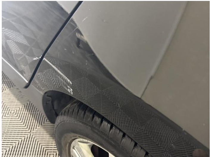
6: Qtr Panel nsr Dented With Paint Damage
