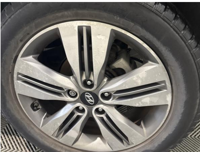
7: Wheel nsr Scratched Over 50mm
