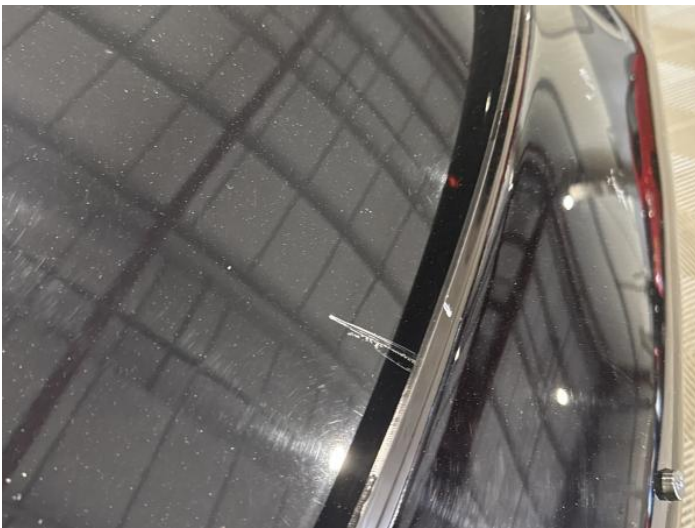
1: Bonnet Scratched Over 25mm Thru Paint
