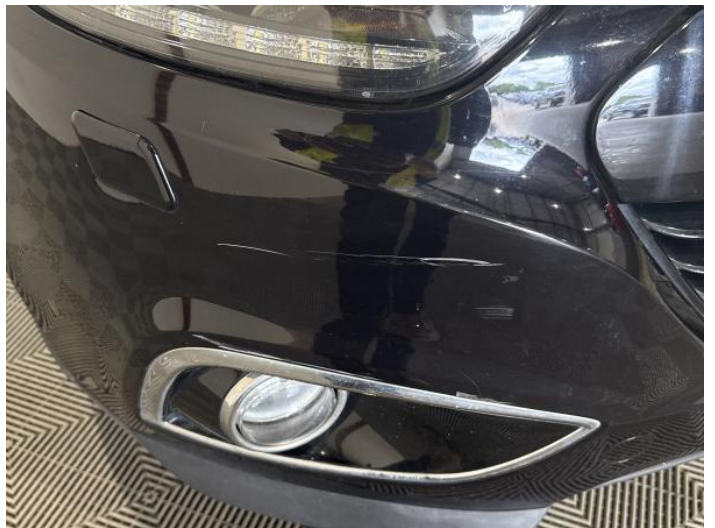
2: Bumper Front Scratched Over 100mm Thru Paint
