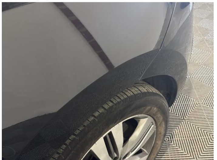
14: Wing osf Scratched Over 25mm Thru Paint
