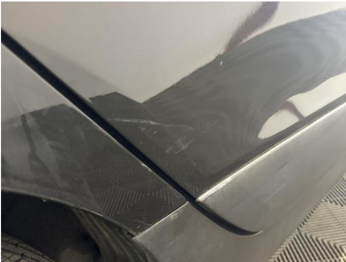
11: Door osr Dented With Paint Damage
