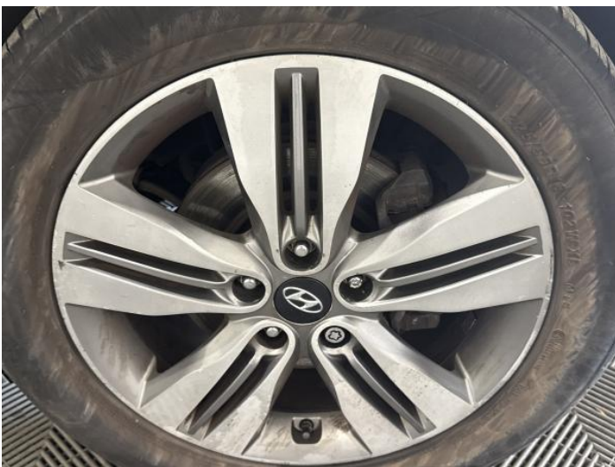
13: Wheel osf Scratched Over 50mm
