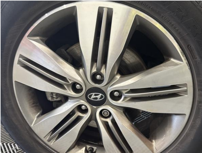
3: Wheel nsf Scratched Up To 50mm
