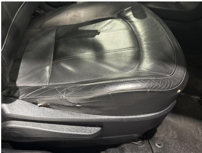
15: Seat Base Cover osf Scuffed Over 25mm
