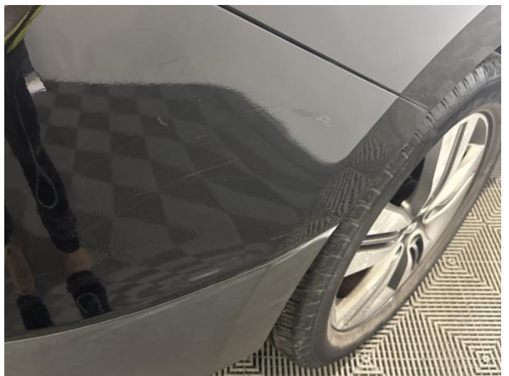
8: Bumper Rear Scratched Over 100mm Thru Paint
