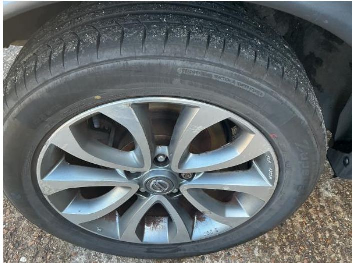
16: Wheel osr Scratched Over 50mm
