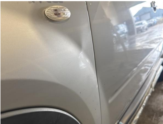
17: Wing nsf Dented Over 30mm
