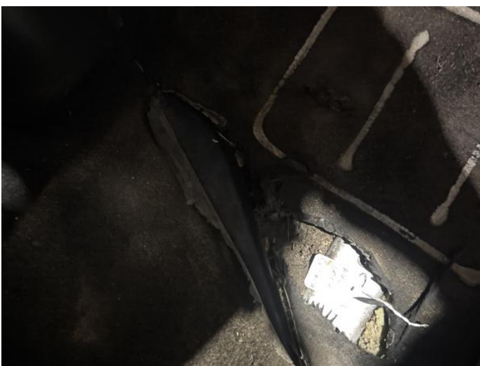
25: Carpets Front Torn Over 10mm
