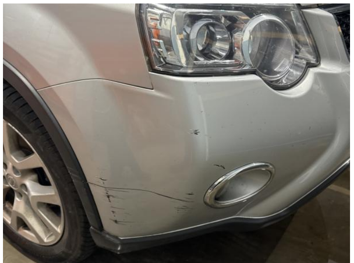
14: Bumper Front Scratched Over 100mm Thru Paint
