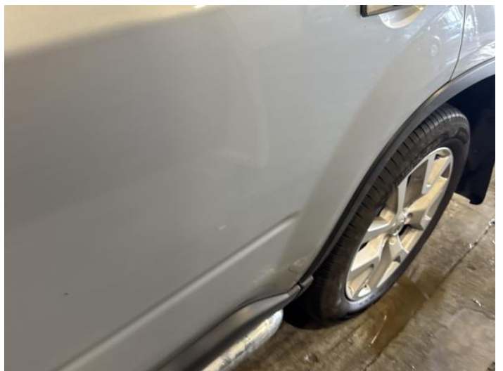
20: Door nsr Dented Over 30mm
