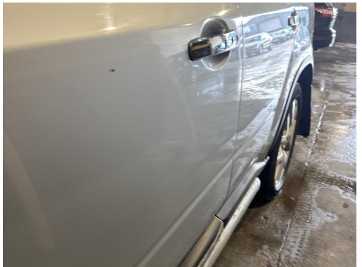
18: Door nsf Dented Over 30mm
