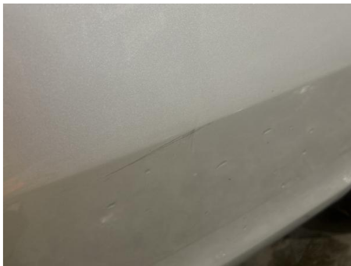
2: Bumper Rear Scratched Over 25mm Not Thru Paint
