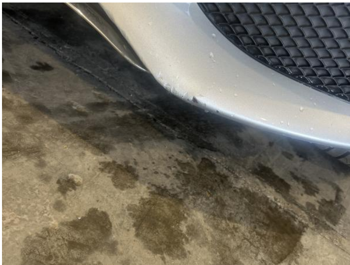
5: Bumper Front Scratched 25 to 100mm Thru Paint
