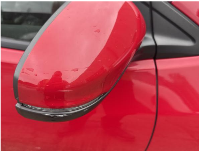
17: Door Mirror Assy osf Scuffed (Unpainted) UpTo 100mm
