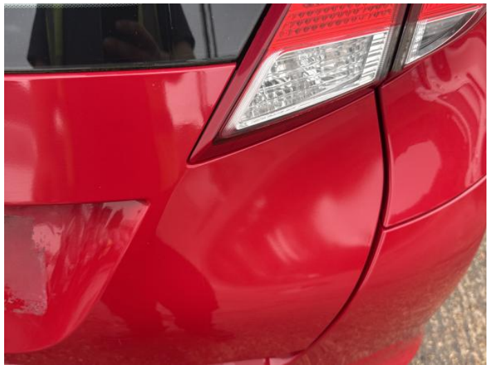
12: Boot Lid Poor Previous Repair Poor Paint
