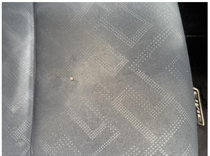
20: Seat Base Cover osf Holed UpTo 3mm
