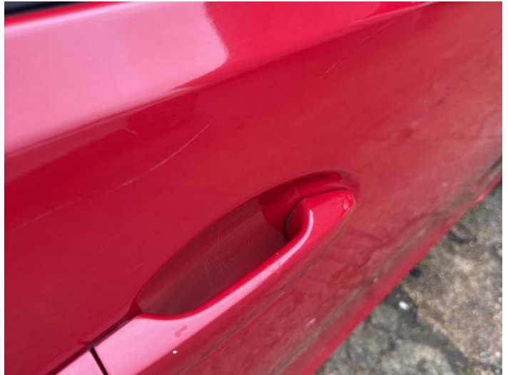
16: Door osf Scratched Over 25mm Thru Paint
