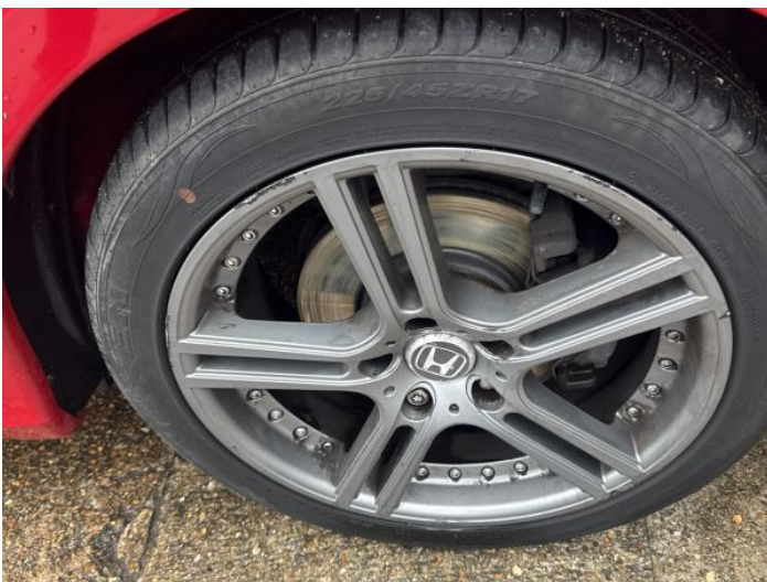
19: Wheel osf Scratched Over 50mm
