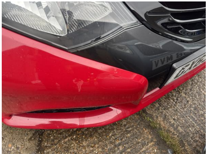
2: Bumper Front Poor Previous Repair Poor Paint
