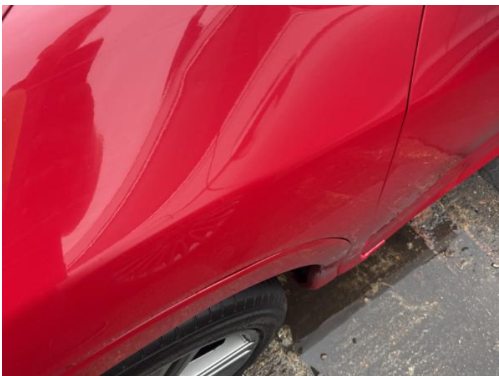
4: Wing nsf Dented Over 2 UpTo 10mm
