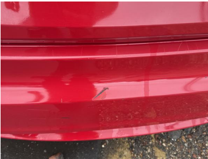
11: Bumper Rear Scratched Over 100mm Thru Paint
