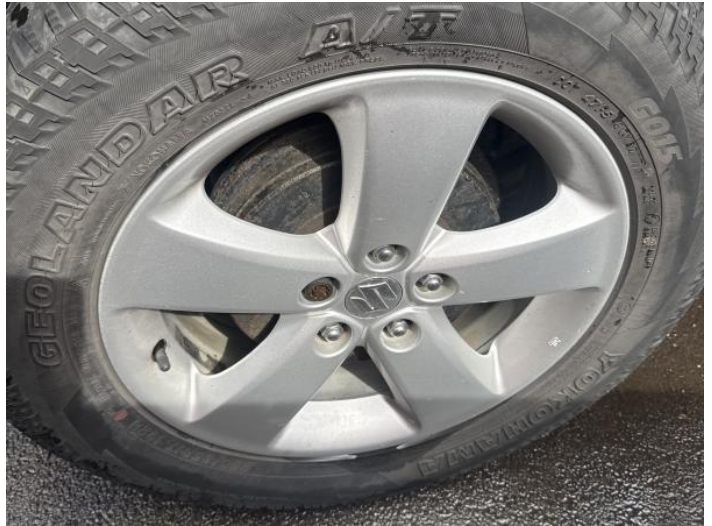
16: Wheel osr Scratched Up To 50mm
