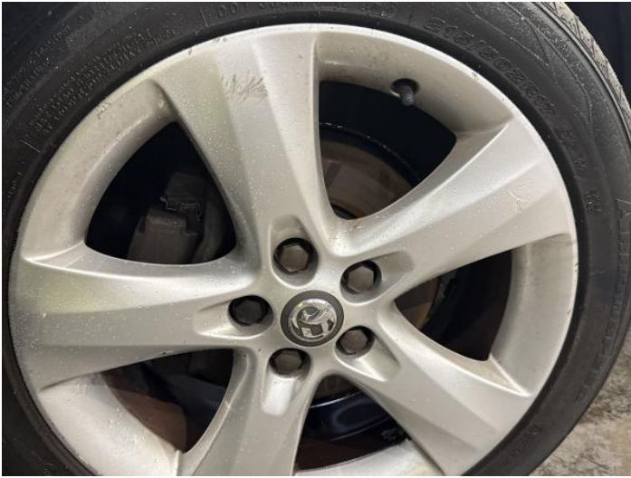
3: Wheel nsf Scratched Over 50mm
