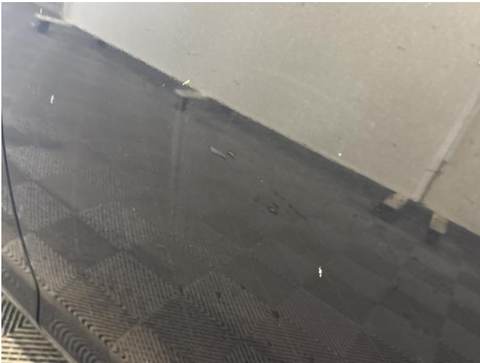
5: Door nsr Scratched Over 25mm Thru Paint
