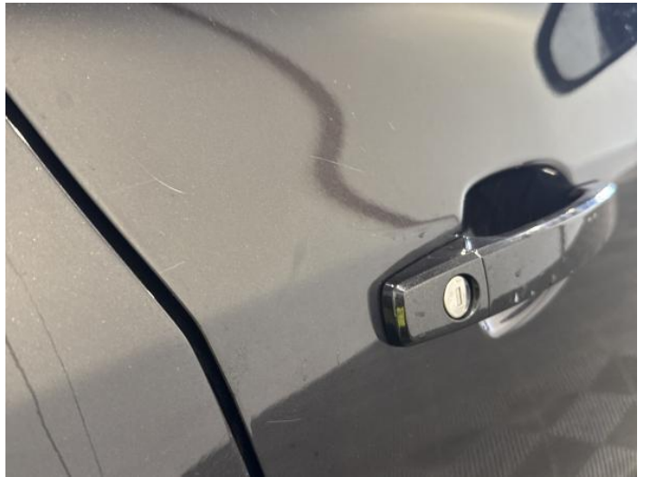
12: Door osf Scratched Over 25mm Thru Paint
