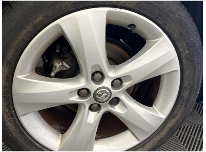
10: Wheel osr Scratched Over 50mm
