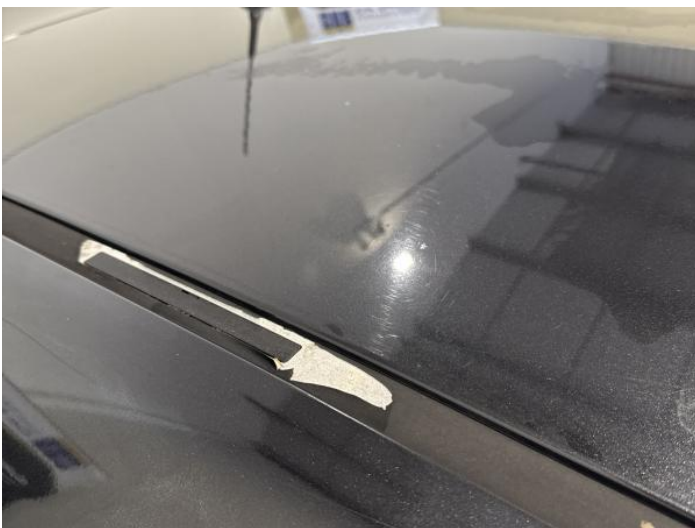
13: Roof Scratched Over 25mm Thru Paint
