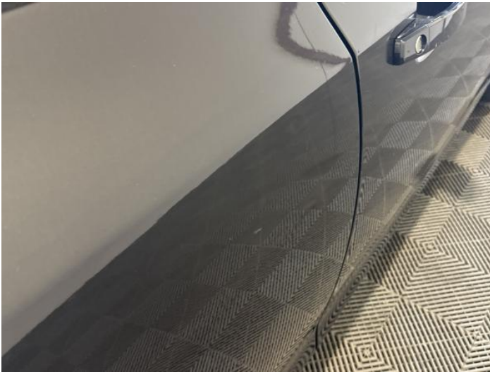
11: Door osr Dented Over 30mm
