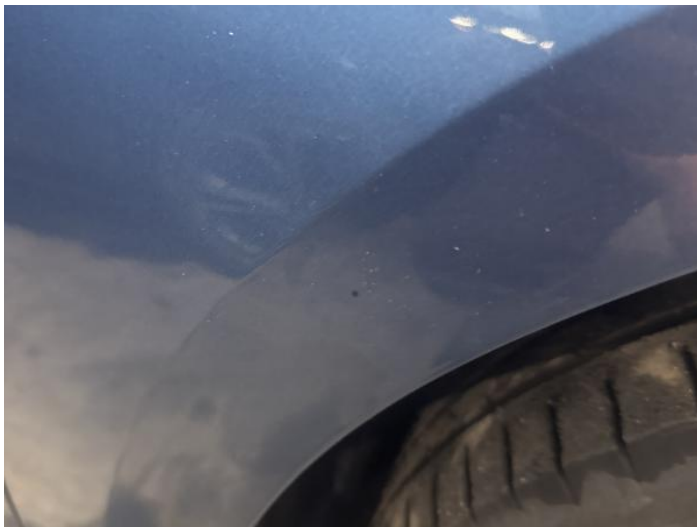
3: Wing osf Dented Between 10mm + 30mm
