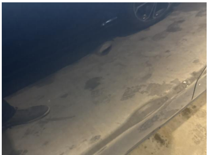
6: Door osr Dented Between 10mm + 30mm
