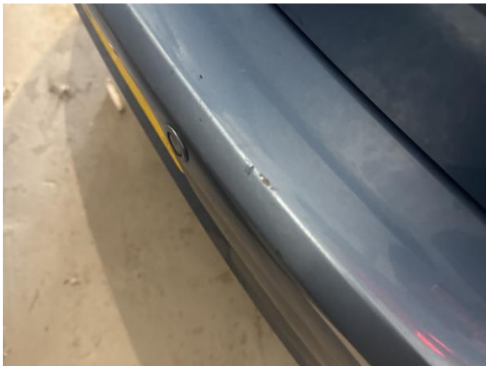
9: Bumper Rear Scratched 25 to 100mm Thru Paint
