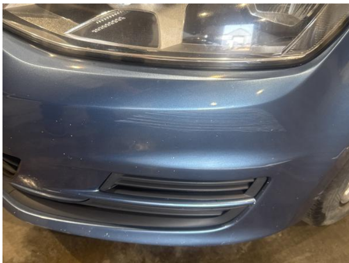
1: Bumper Front Scratched Over 100mm Thru Paint
