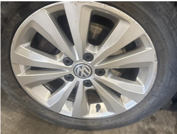
17: Wheel nsf Scratched Over 50mm
