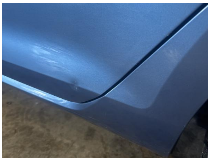
14: Door nsr Dented With Paint Damage
