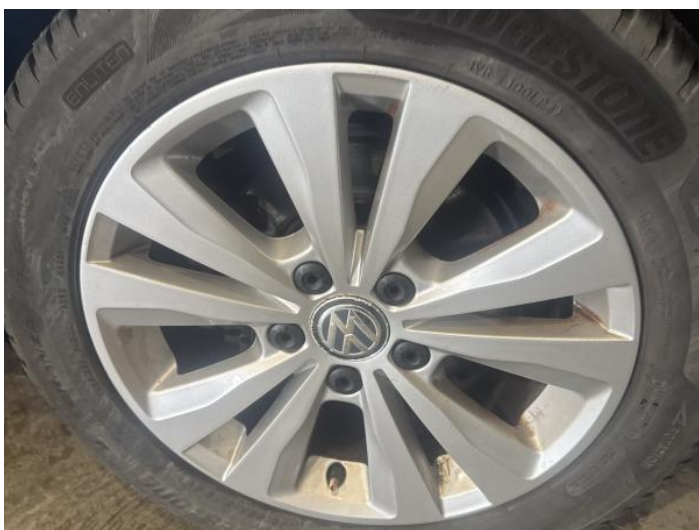
13: Wheel nsr Scratched Up To 50mm
