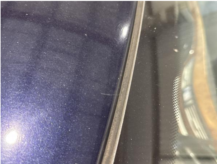
17: Roof Scratched UpTo 25mm Thru Paint
