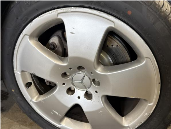
15: Wheel osf Scratched Over 50mm
