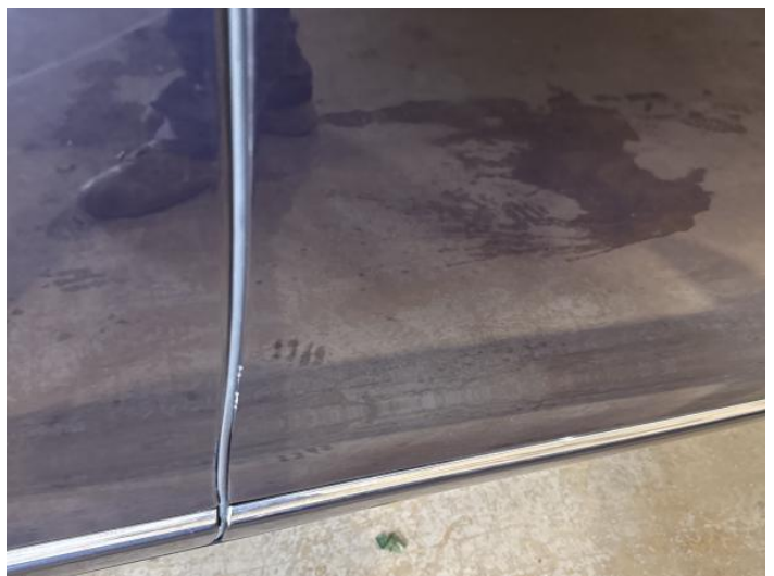
14: Door osf Scratched Over 25mm Thru Paint
