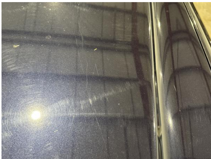
1: Bonnet Scratched Over 25mm Thru Paint
