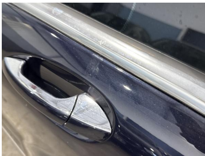
8: Door nsr Scratched UpTo 25mm Thru Paint
