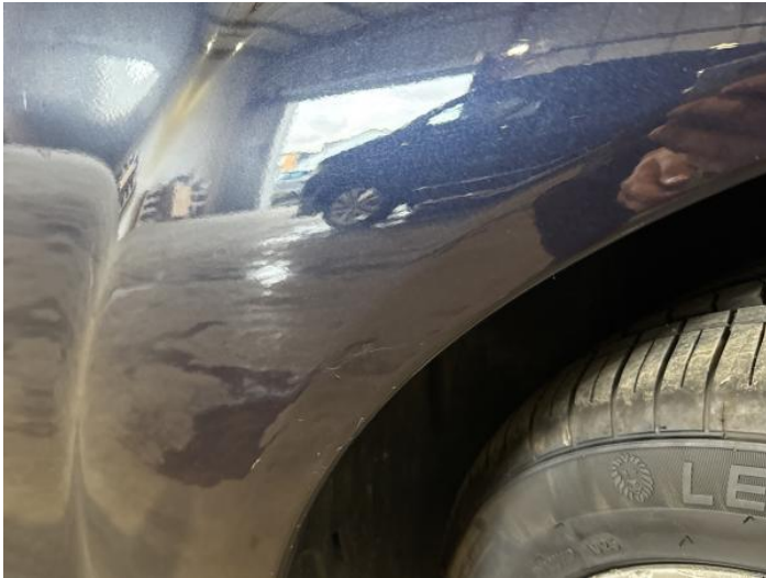
16: Wing osf Scratched UpTo 25mm Thru Paint
