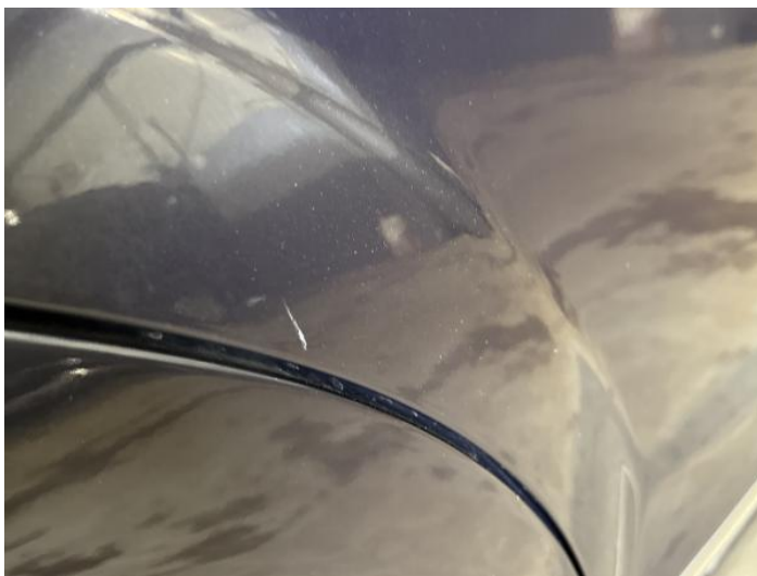
13: Door osr Scratched Over 25mm Thru Paint
