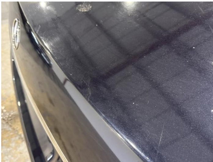
11: Boot Lid Scratched Over 25mm Thru Paint
