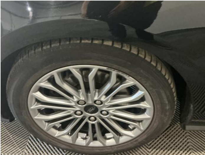
3: Wheel nsf Scratched Over 50mm
