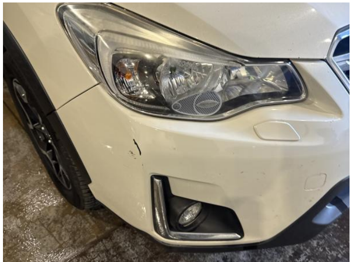
2: Bumper Front Scratched Over 100mm Thru Paint
