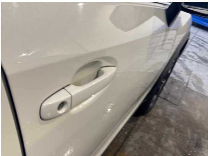
15: Door osf Dented Over 2 UpTo 10mm
