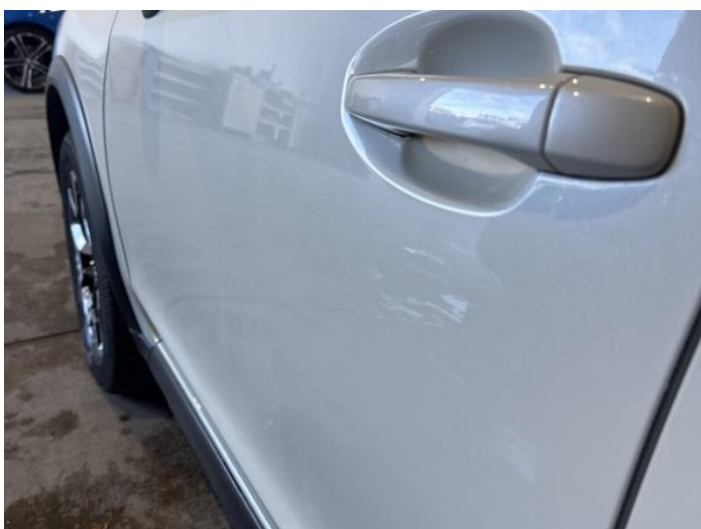
5: Door nsf Dented Over 2 UpTo 10mm
