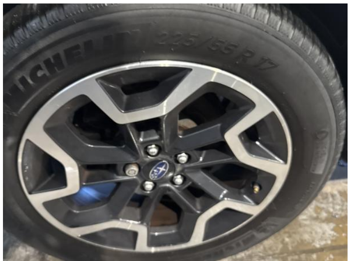
14: Wheel osr Scratched Up To 50mm
