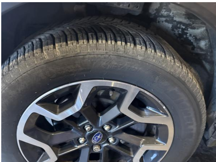
3: Wheel nsf Scratched Over 50mm
