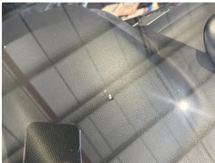
18: Screen Front Chipped UpTo 10mm
