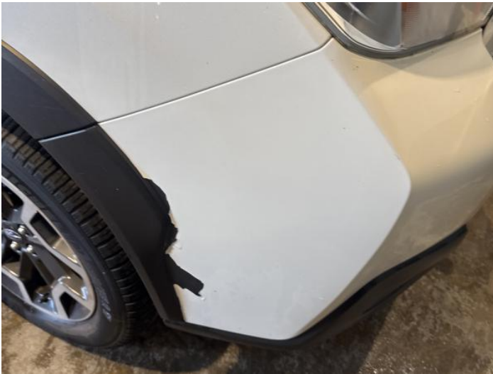
11: Bumper Rear Poor Previous Repair Paint Flake
