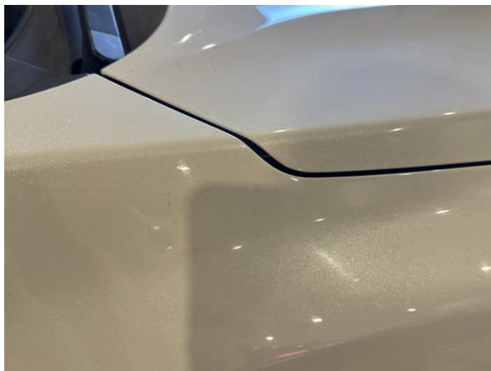
16: Wing osf Chipped 1 To 5
