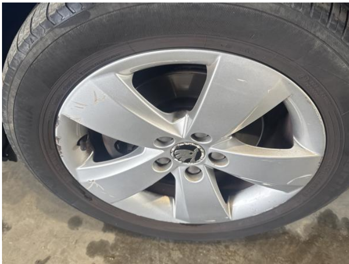
15: Wheel nsf Scratched Over 50mm
