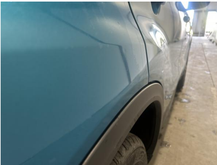
5: Qtr Panel osr Dented 2 Or Less UpTo 10mm
