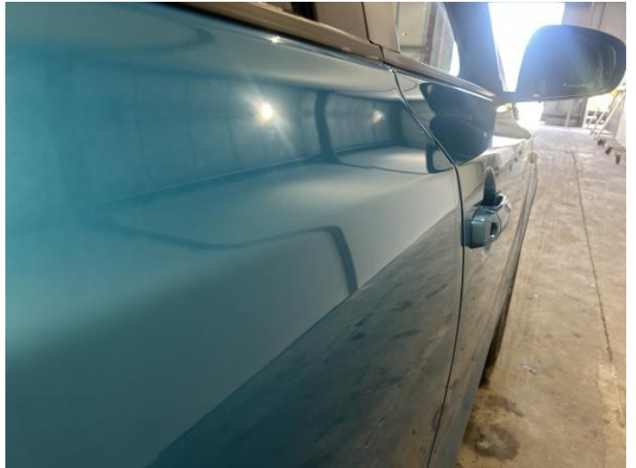
4: Door osr Dented 2 Or Less UpTo 10mm
