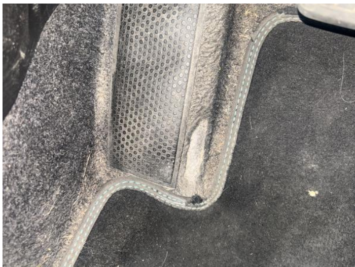
1: Carpets Front Torn Between 3mm + 10mm
