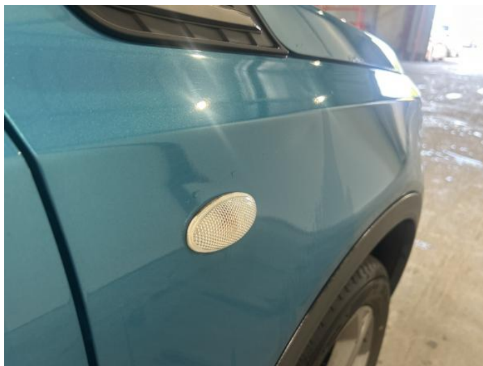
2: Wing osf Dented Over 30mm
