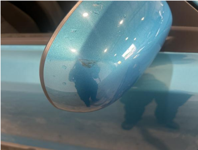
3: Door Mirror Assy osf Scratched (Painted) UpTo 25mm Thru Paint
