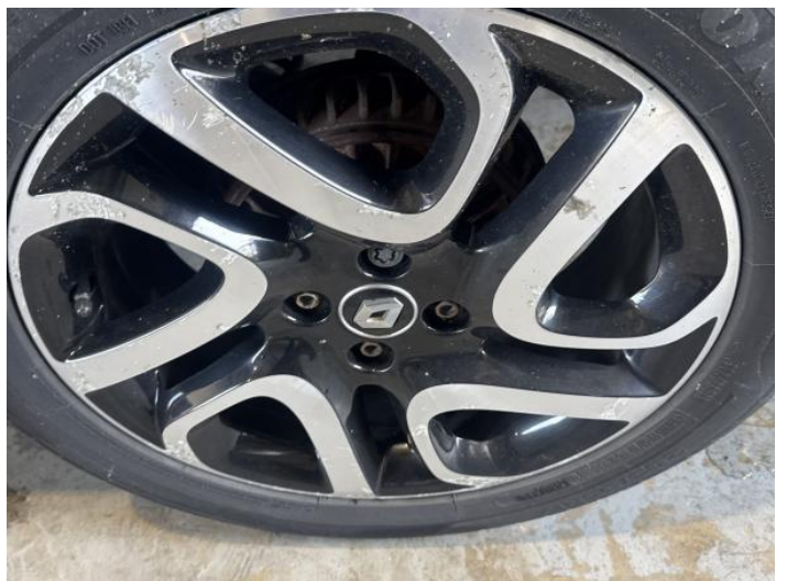
8: Wheel nsr Corroded Light
