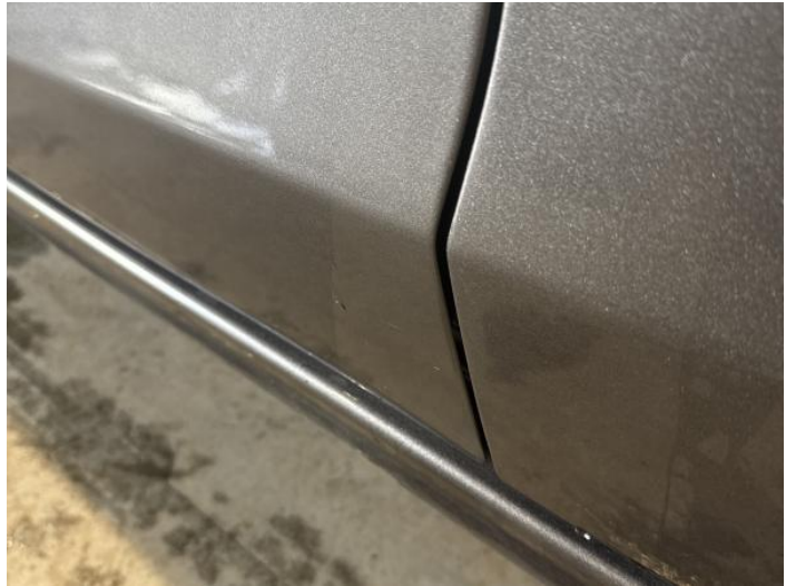
4: Door nsf Scratched UpTo 25mm Thru Paint
