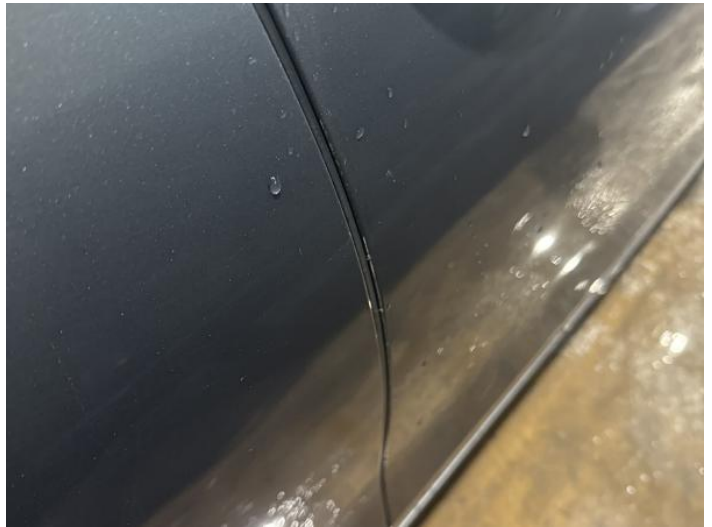
12: Door osr Scratched UpTo 25mm Thru Paint
