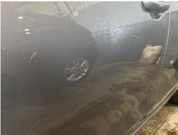
5: Door nsf Scratched Over 25mm Thru Paint
