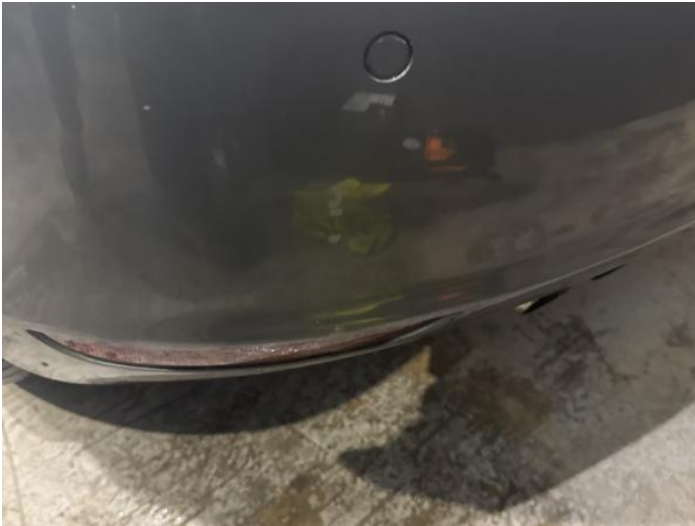
9: Bumper Rear Scratched 25 to 100mm Thru Paint
