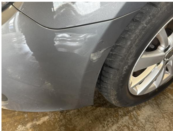
2: Bumper Front Dented With Paint Damage
