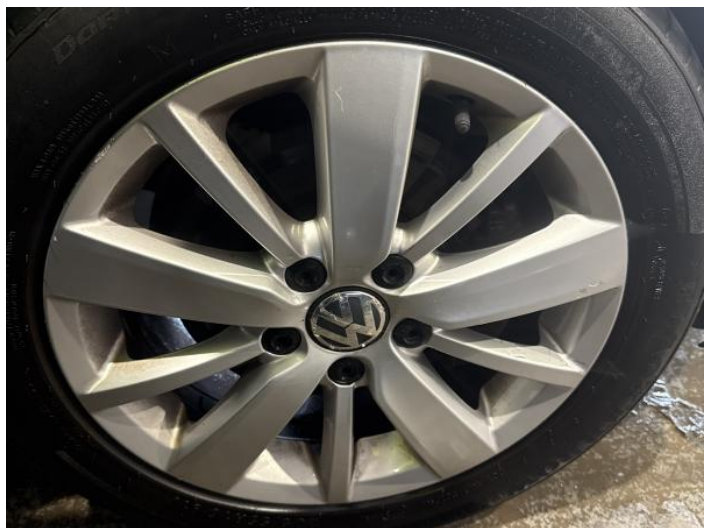
14: Wheel osf Scratched Over 50mm
