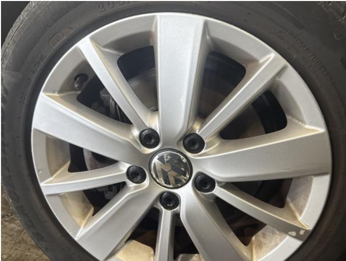
3: Wheel nsf Scratched Over 50mm
