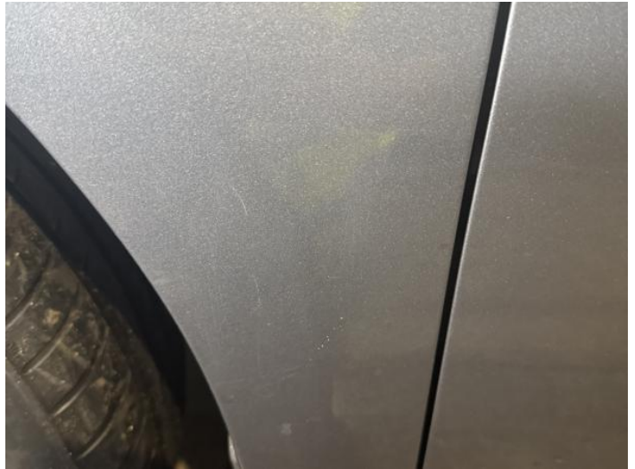
4: Wing nsf Scratched UpTo 25mm Thru Paint
