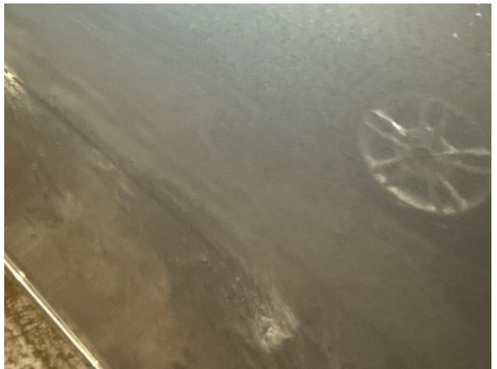
6: Door nsr Scratched UpTo 25mm Thru Paint
