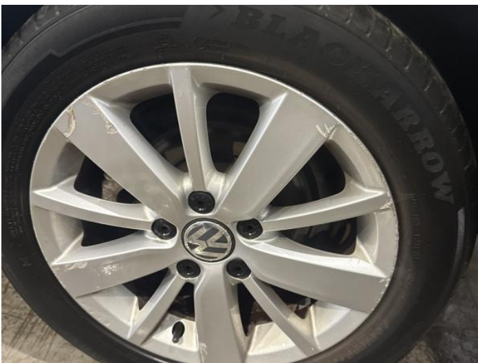
7: Wheel nsr Scratched Over 50mm
