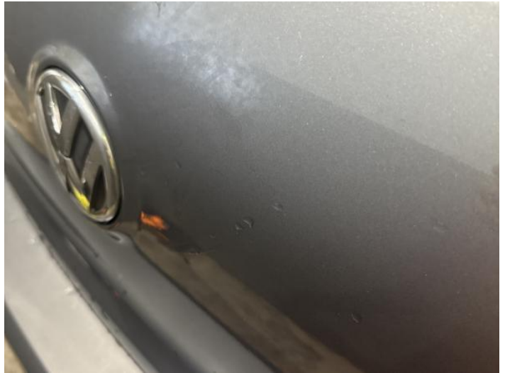
10: Tailgate Scratched UpTo 25mm Thru Paint
