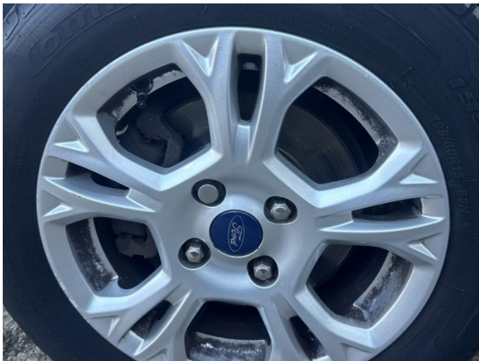
3: Wheel nsf Scratched Over 50mm
