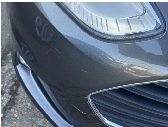
2: Bumper Front Scratched Over 100mm Thru Paint
