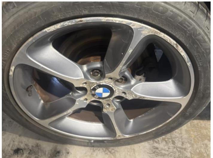
6: Wheel osr Scratched Over 50mm
