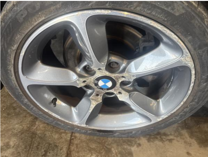
12: Wheel nsf Scratched Over 50mm
