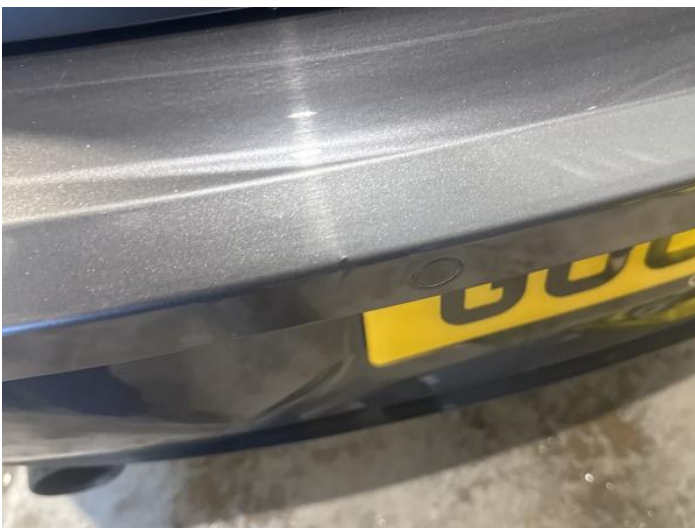
7: Bumper Rear Chipped Multiple Chips
