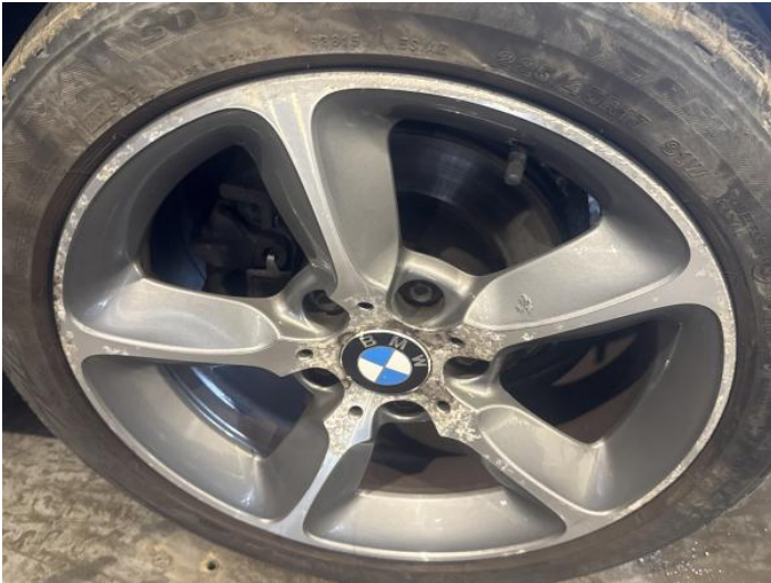
3: Wheel osf Scratched Over 50mm
