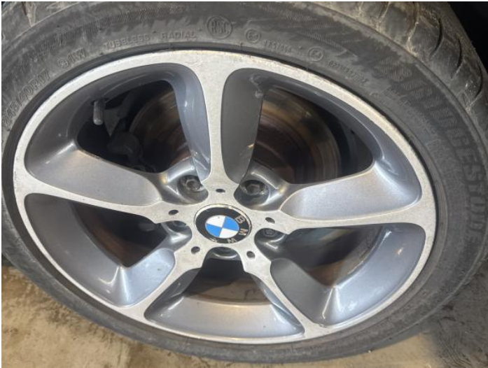
9: Wheel nsr Scratched Over 50mm
