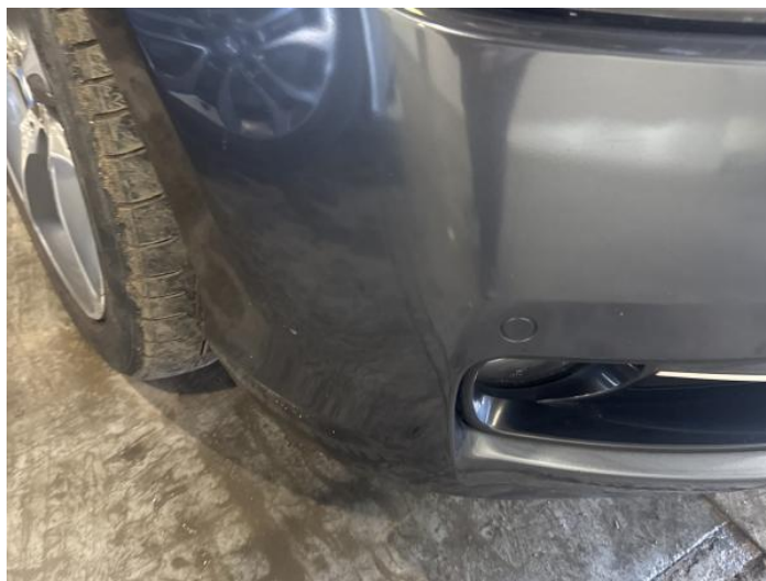
2: Bumper Front Scratched Over 100mm Thru Paint
