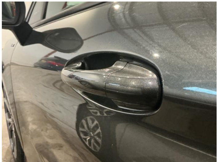
6: Door nsf Dented Between 10mm + 30mm
