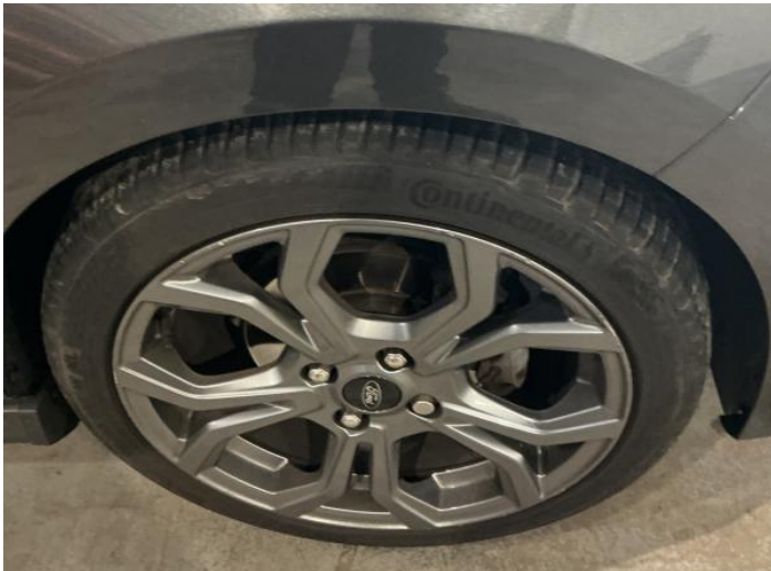
18: Wheel osf Scratched Up To 50mm
