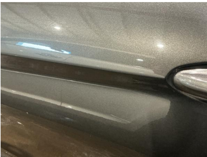
7: Door nsr Scratched UpTo 25mm Thru Paint
