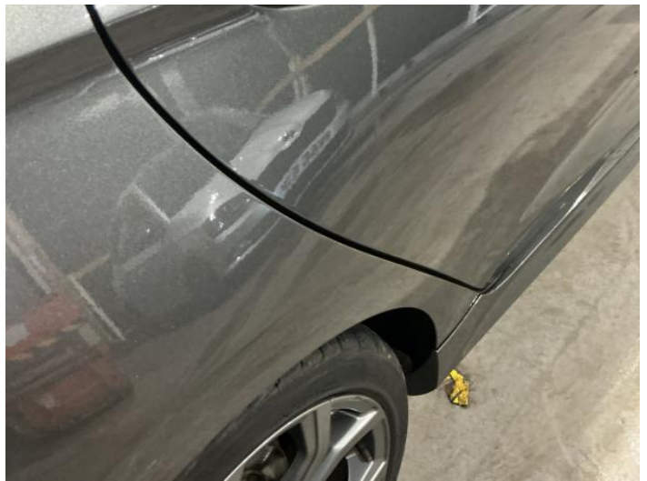
12: Qtr Panel osr Dented 2 Or Less UpTo 10mm
