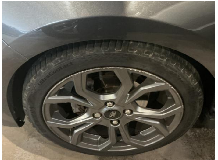
4: Wheel nsf Scratched Over 50mm
