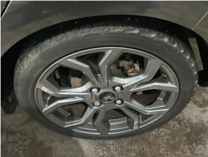
9: Wheel nsr Scratched Up To 50mm
