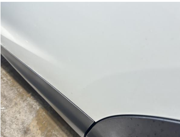
7: Door nsr Dented Between 10mm + 30mm
