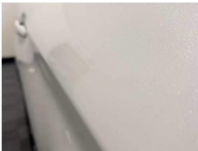
20: Door osr Dented Over 2 UpTo 10mm
