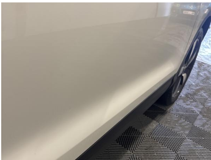
17: Door osf Dented Between 10mm + 30mm
