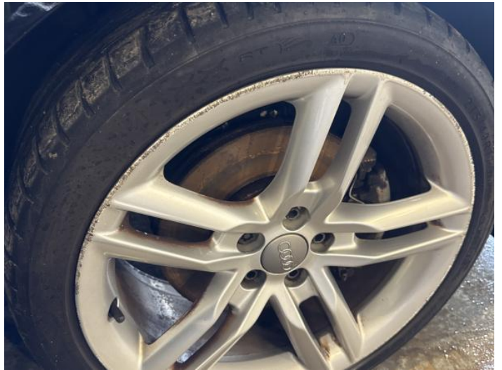
12: Wheel osf Scratched Over 50mm
