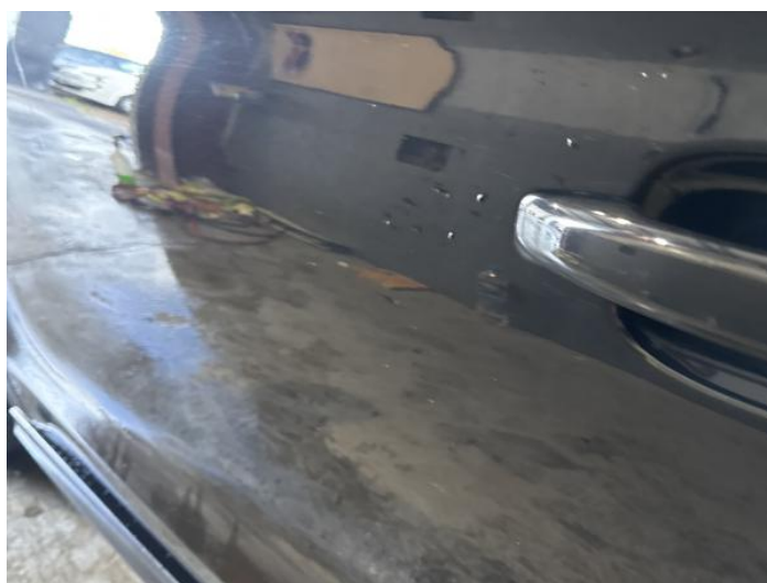
6: Door nsf Poor Previous Repair Poor Paint
