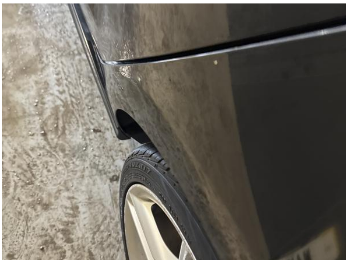
3: Qtr Panel nsf Dented Over 2 UpTo 10mm
