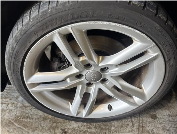
9: Wheel nsf Scratched Over 50mm
