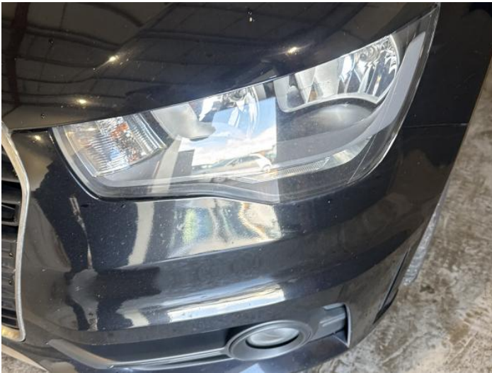
11: Bumper Front Poor Previous Repair Poor Paint
