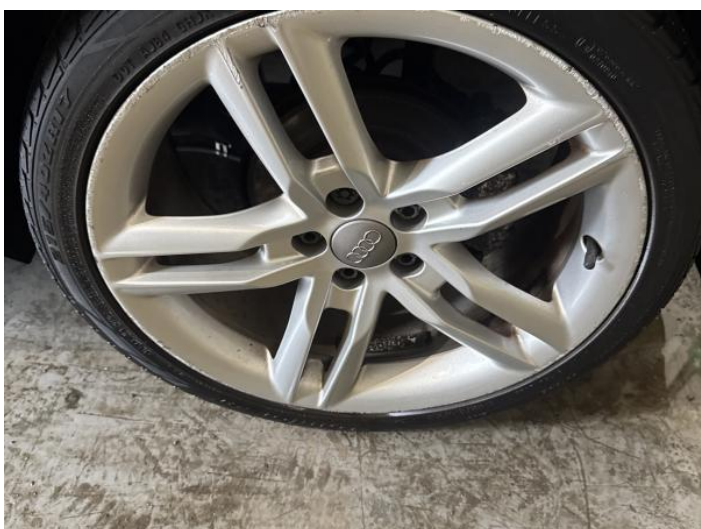
5: Wheel nsf Scratched Over 50mm
