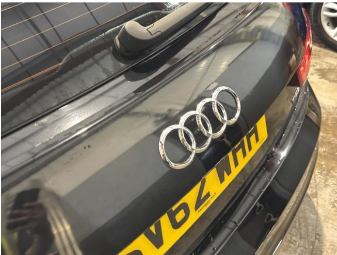
1: Boot Lid Poor Previous Repair Poor Paint
