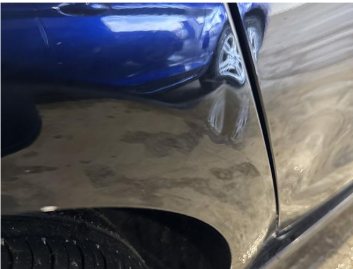
17: Qtr Panel osr Dented Between 10mm + 30mm
