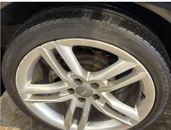
19: Wheel osf Scratched Over 50mm
