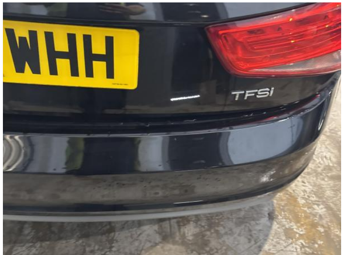
2: Bumper Rear Poor Previous Repair Poor Paint
