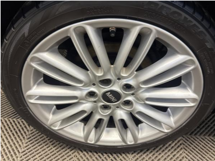
9: Wheel osr Corroded Light
