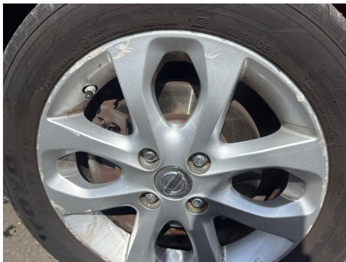
4: Wheel nsf Scratched Over 50mm
