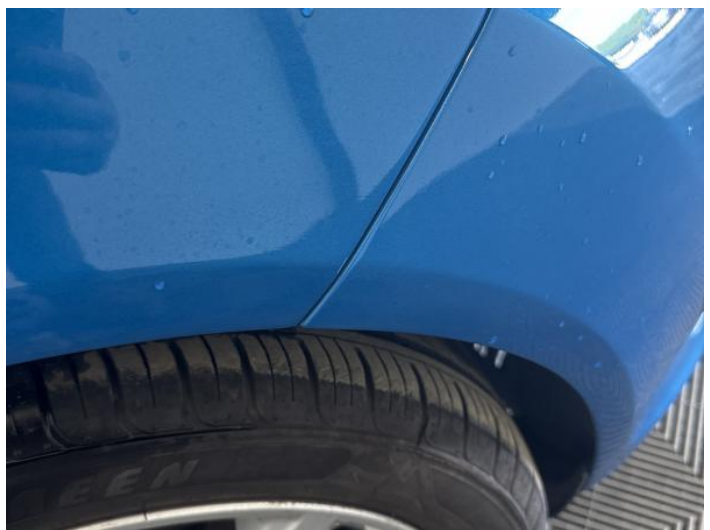
12: Wing osf Scratched UpTo 25mm Thru Paint
