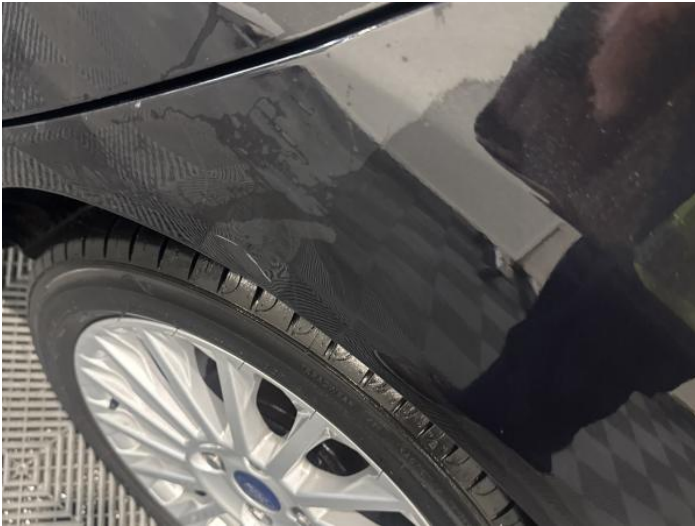
9: Qtr Panel nsr Dented With Paint Damage
