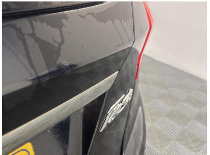
12: Boot Lid Dented Between 10mm + 30mm
