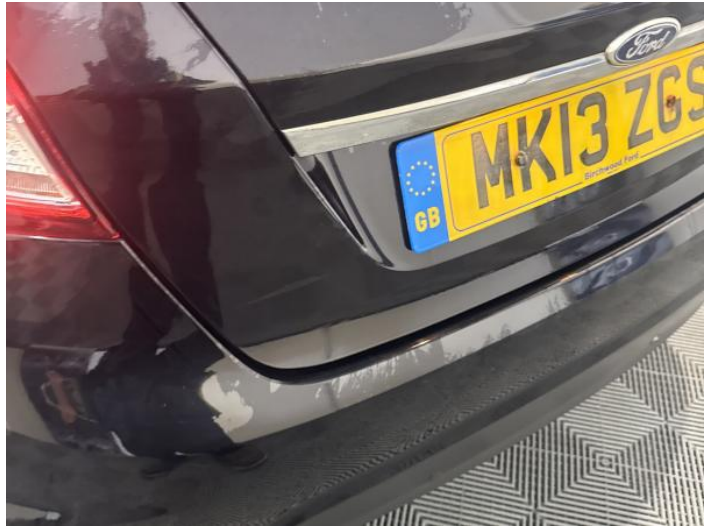
10: Bumper Rear Chipped Multiple Chips
