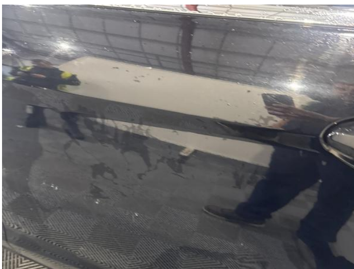
7: Door nsr Chipped Multiple Chips
