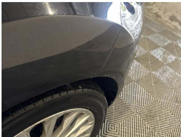
18: Wing osf Dented Between 10mm + 30mm
