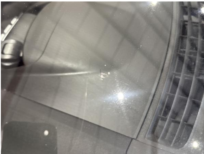
22: Screen Front Chipped UpTo 10mm
