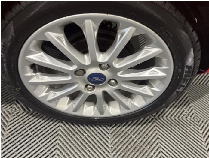
11: Wheel nsr Scratched Up To 50mm
