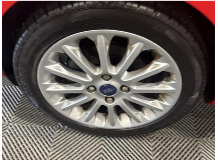
4: Wheel nsf Scratched Up To 50mm
