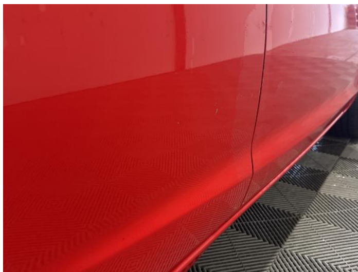
18: Door osr Chipped Multiple Chips
