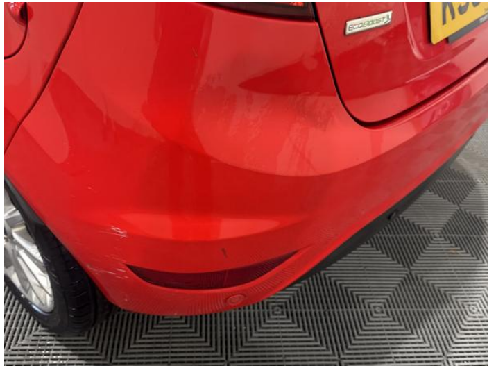
12: Bumper Rear Scratched 25 to 100mm Thru Paint
