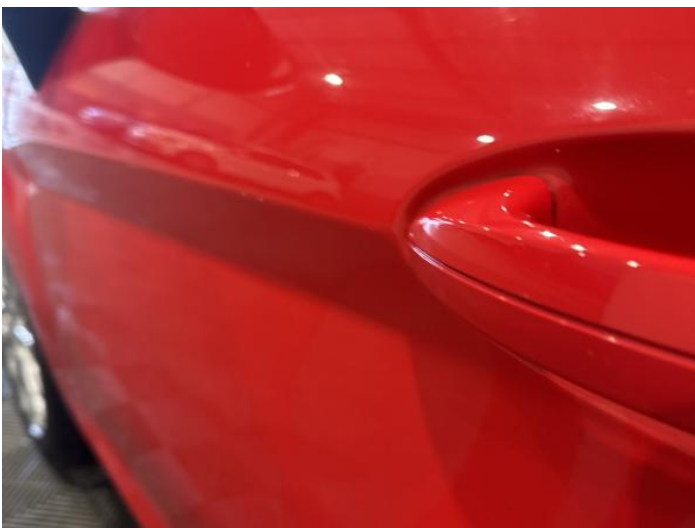
7: Door nsf Dented With Paint Damage
