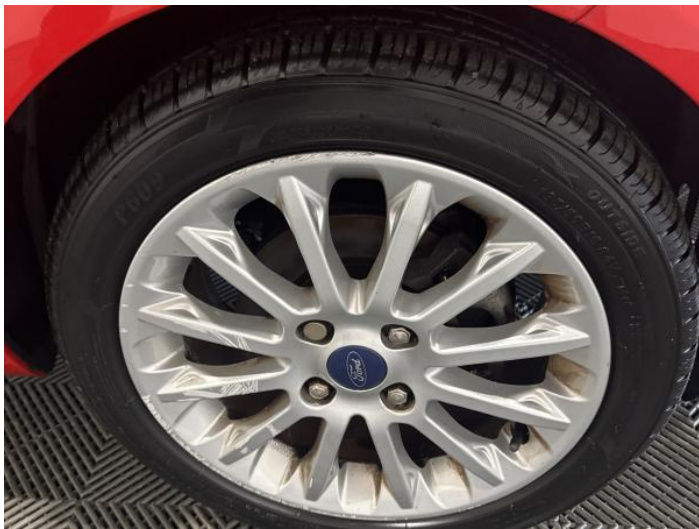
23: Wheel osf Scratched Over 50mm
