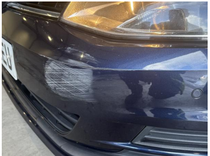
2: Bumper Front Scratched Over 100mm Thru Paint
