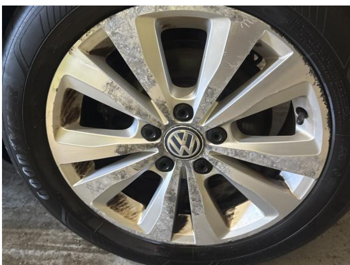
7: Wheel nsr Scratched Over 50mm
