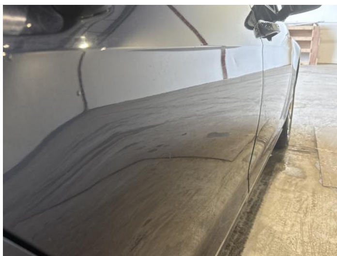
12: Door osr Dented Over 30mm
