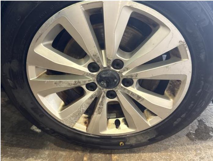
15: Wheel osf Scratched Over 50mm
