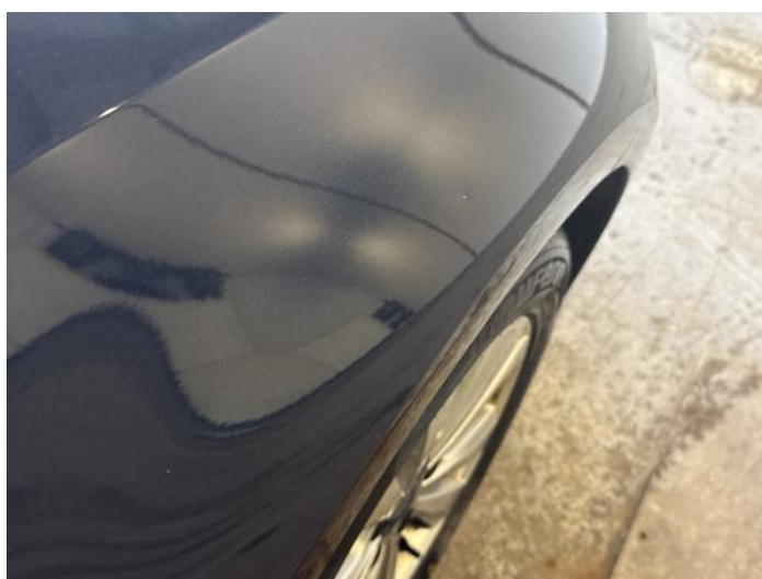
14: Wing osf Dented Between 10mm + 30mm
