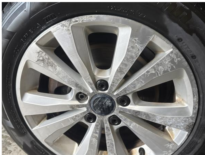
4: Wheel nsf Scratched Over 50mm
