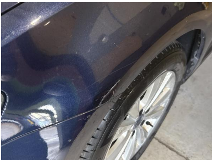
3: Wing nsf Dented With Paint Damage
