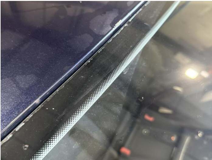
17: Roof Chipped Edge Chip
