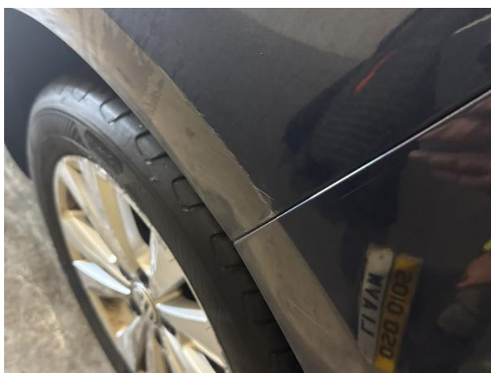
8: Qtr Panel nsr Dented With Paint Damage
