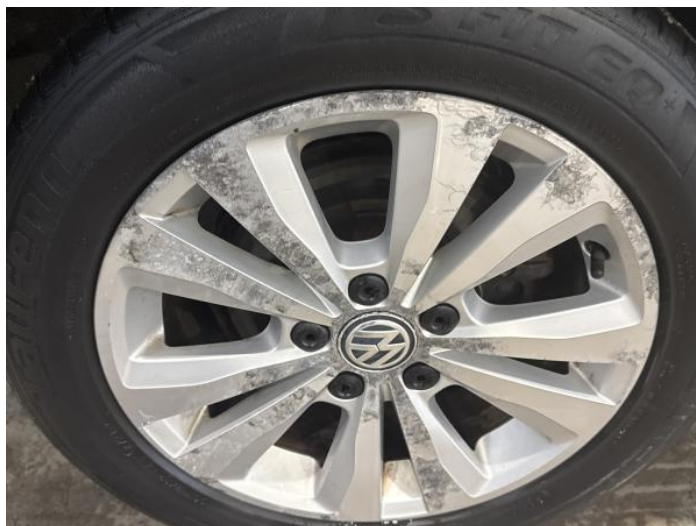
10: Wheel osr Scratched Over 50mm
