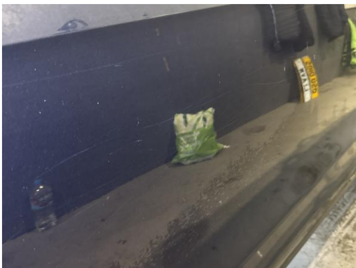
5: Door nsf Scratched Over 25mm Thru Paint
