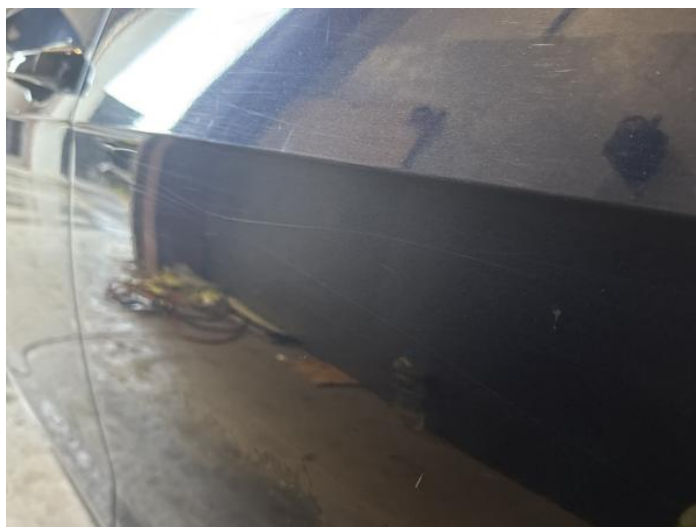
6: Door nsr Scratched Over 25mm Thru Paint
