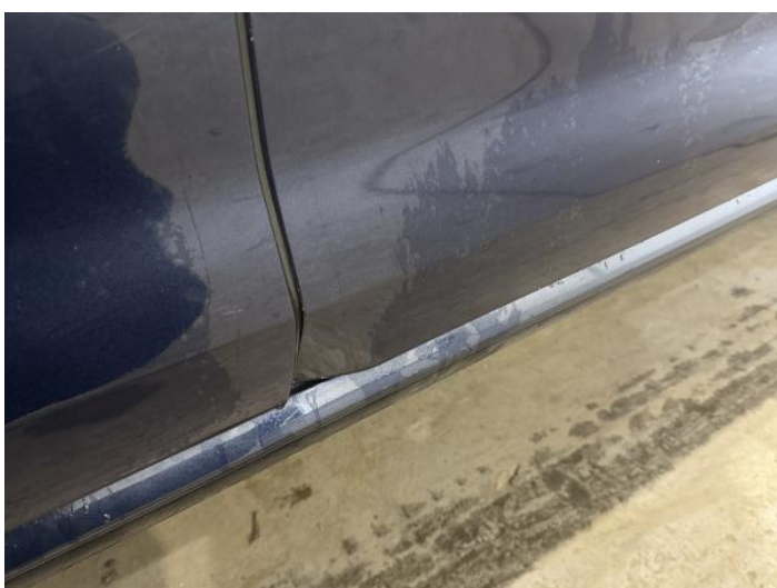
13: Door osf Dented Over 30mm
