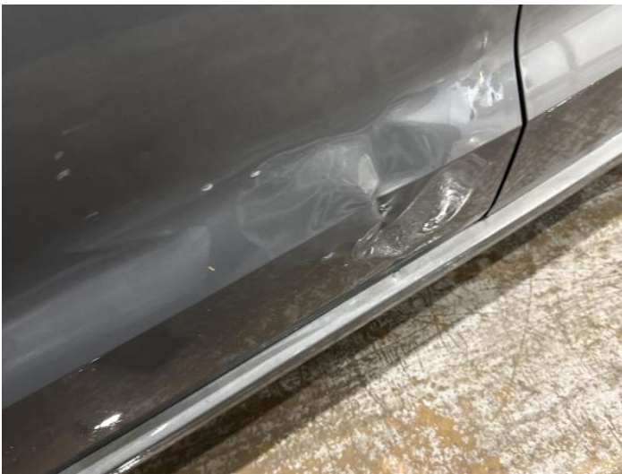
5: Door nsf Dented Over 30mm
