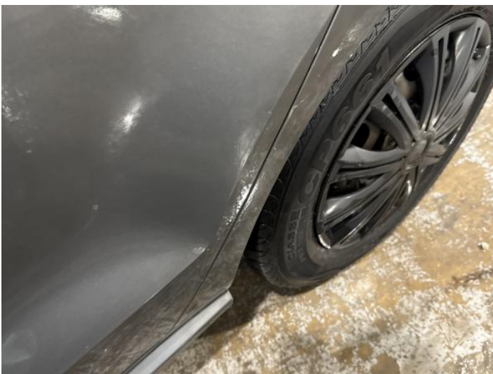
7: Door nsr Scratched Over 25mm Thru Paint
