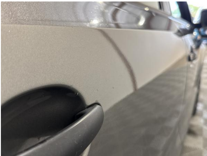
12: Door osr Dented Between 10mm + 30mm
