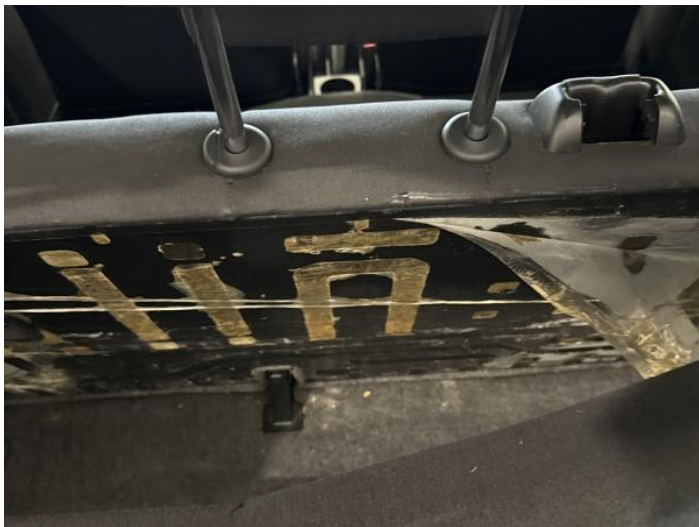
15: Seat Back Cover osr Scuffed Over 25mm
