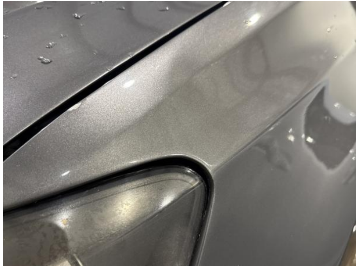
4: Wing nsf Dented Over 30mm
