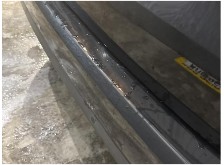
10: Bumper Rear Scratched 25 to 100mm Thru Paint
