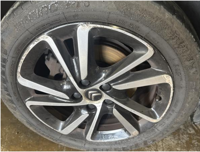
3: Wheel nsf Scratched Over 50mm
