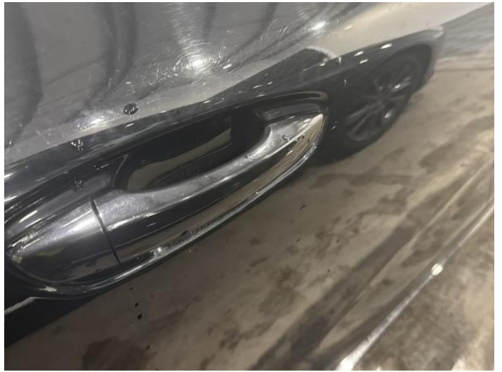
12: Door osr Scratched Over 25mm Thru Paint
