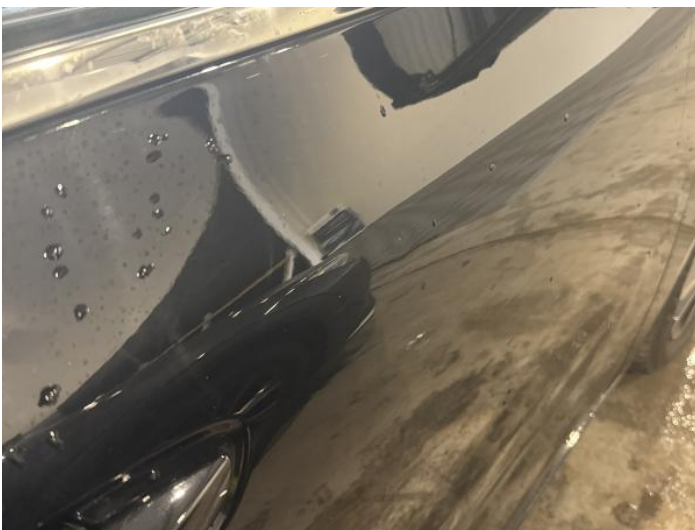
13: Door osf Dented Between 10mm + 30mm
