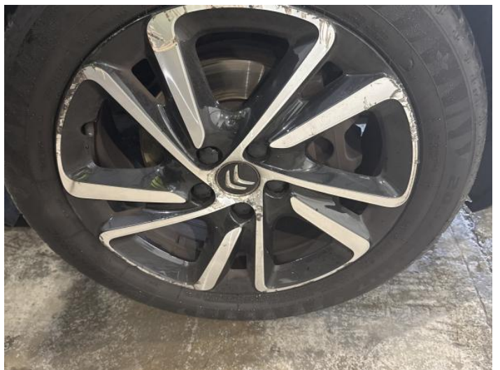
14: Wheel nsf Scratched Over 50mm
