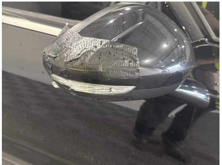
16: Door Mirror Assy osf Broken Replace
