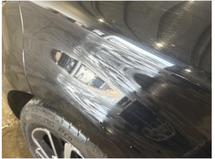
4: Wing nsf Scratched Over 25mm Thru Paint
