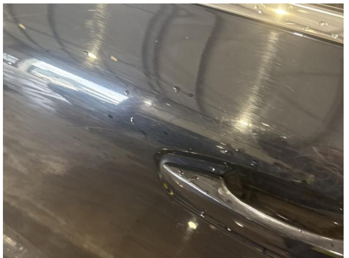
8: Door nsr Scratched Over 25mm Thru Paint
