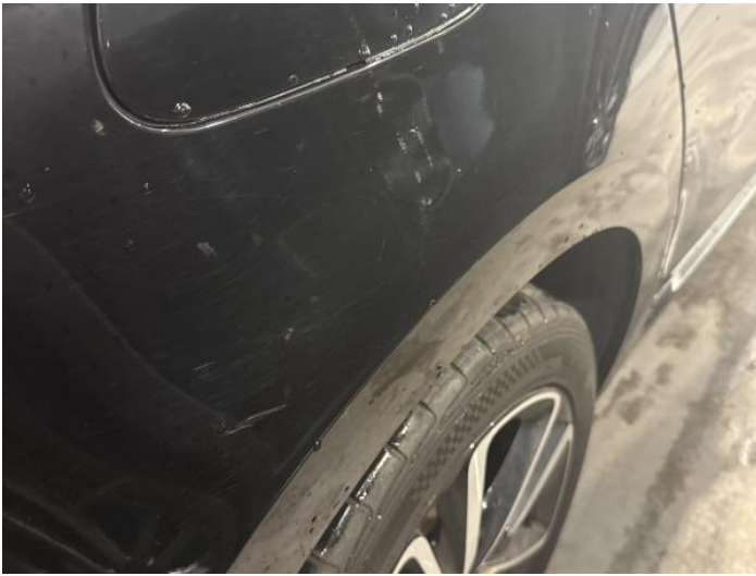
11: Qtr Panel osr Dented With Paint Damage
