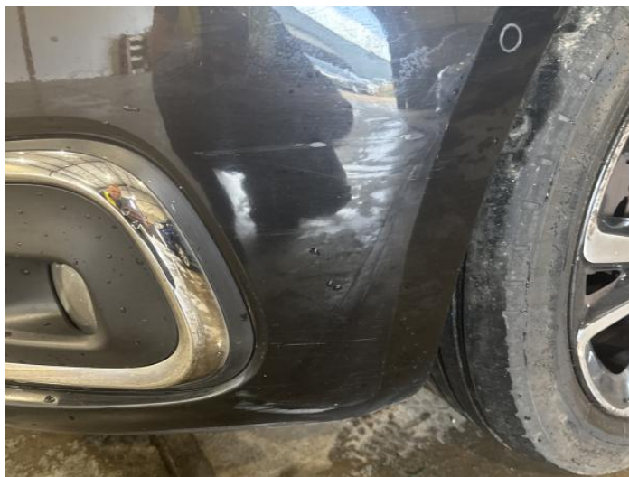
2: Bumper Front Scratched Over 100mm Thru Paint
