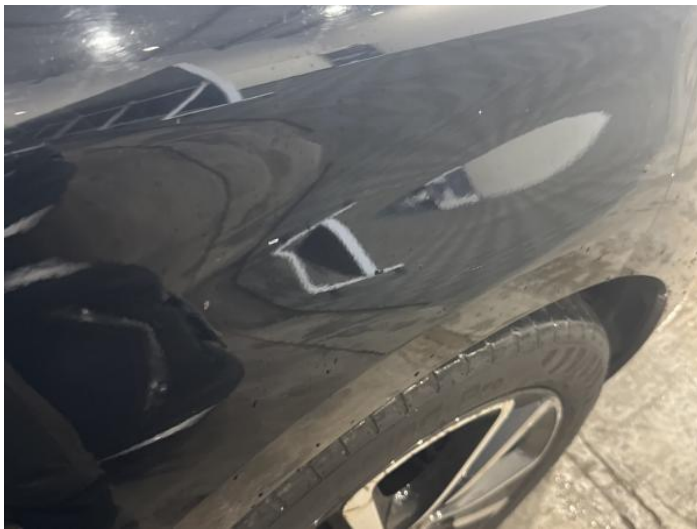
15: Wing osf Scratched UpTo 25mm Thru Paint
