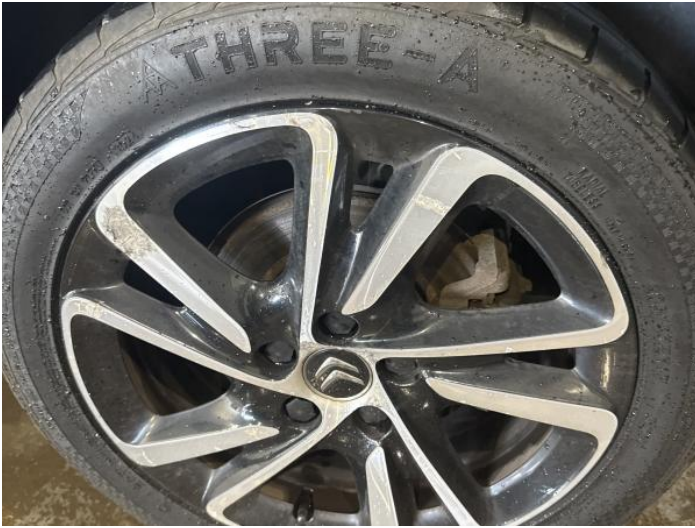
9: Wheel nsr Scratched Over 50mm
