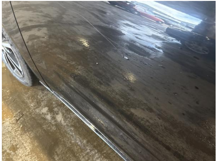
6: Door nsf Scratched Over 25mm Thru Paint
