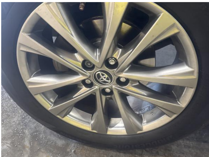
13: Wheel nsf Scratched Up To 50mm
