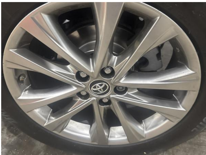
9: Wheel nsr Scratched Up To 50mm
