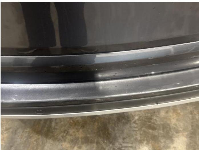
7: Bumper Rear Chipped Multiple Chips
