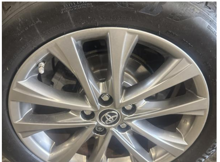
6: Wheel osr Scratched Up To 50mm
