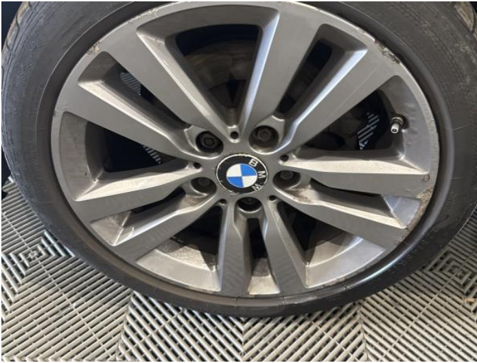
3: Wheel nsf Scratched Over 50mm
