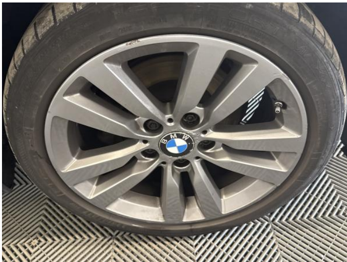
11: Wheel osf Scratched Over 50mm
