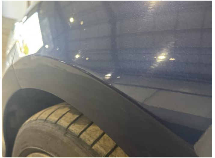
4: Wing nsf Dented Over 30mm
