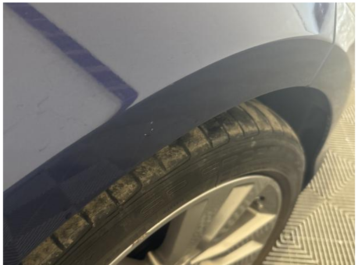
10: Wing osf Dented Over 30mm
