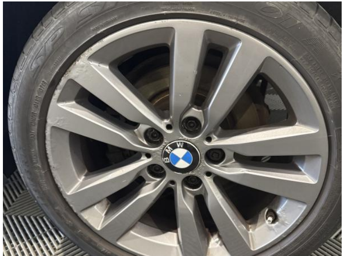
6: Wheel nsr Scratched Over 50mm
