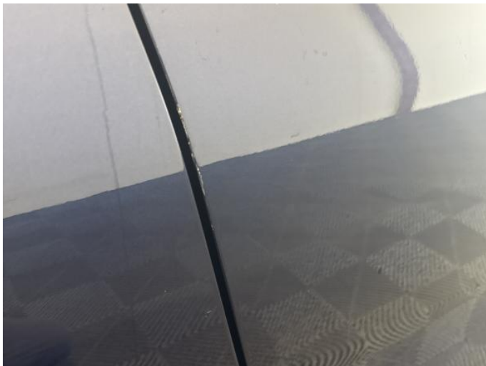
9: Door osf Chipped Edge Chip
