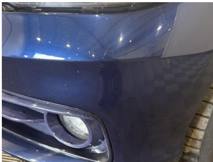
2: Bumper Front Scratched 25 to 100mm Thru Paint
