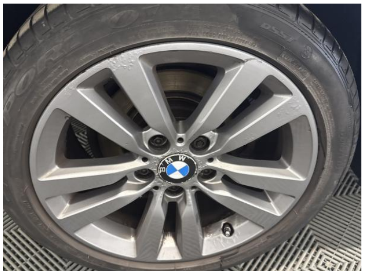
8: Wheel osr Scratched Over 50mm
