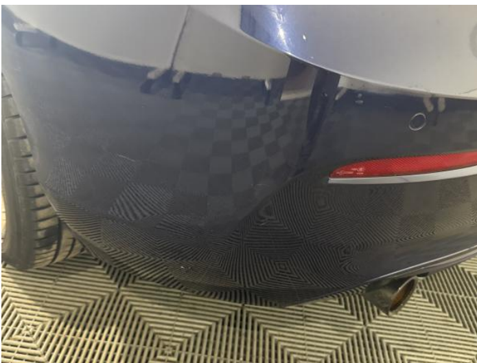
7: Bumper Rear Scratched 25 to 100mm Thru Paint
