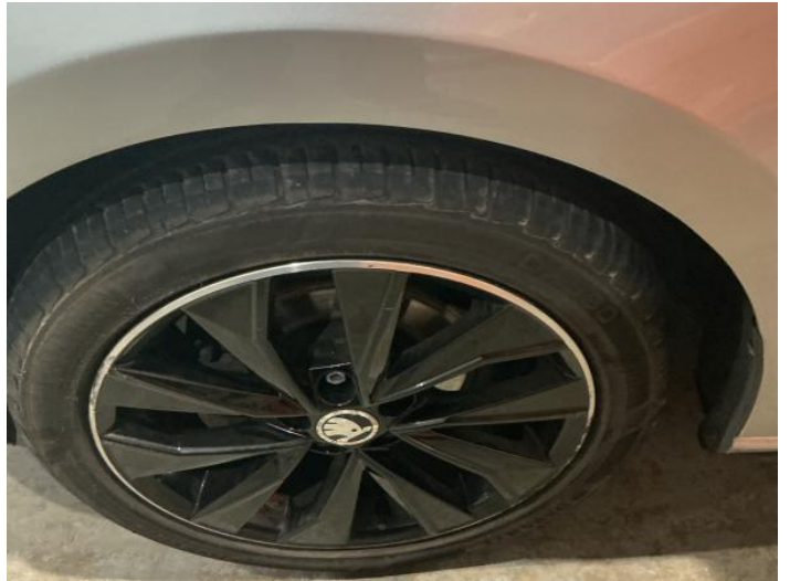
4: Wheel nsf Scratched Over 50mm
