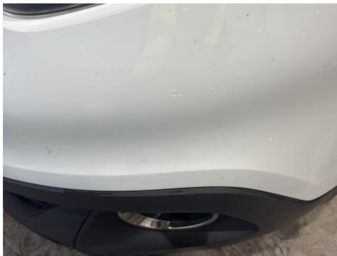
2: Bumper Front Scratched 25 to 100mm Thru Paint
