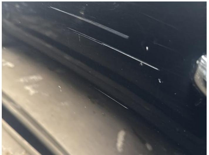
6: Door nsr Scratched Over 25mm Thru Paint
