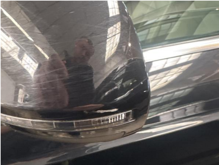
9: Door Mirror Assy nsf Scratched (Painted) Over 25mm Thru Paint
