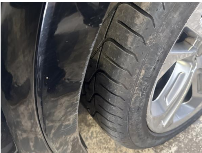
13: Wing Front Arch Extension nsf Scratched (Painted) Over 25mm Thru Paint
