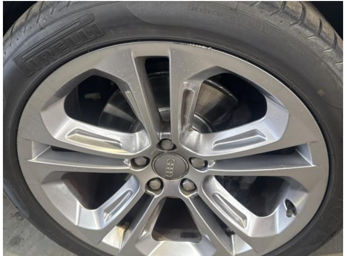
16: Wheel osf Scratched Up To 50mm
