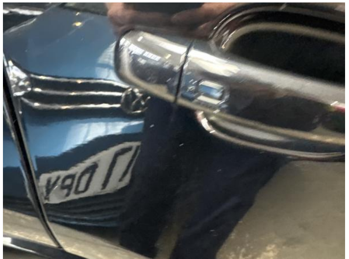
18: Door osr Scratched Over 25mm Not Thru Paint
