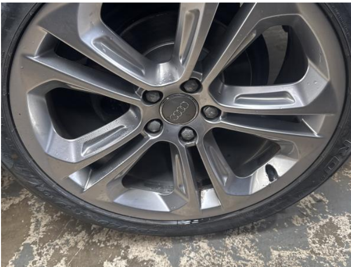
5: Wheel nsr Scratched Up To 50mm
