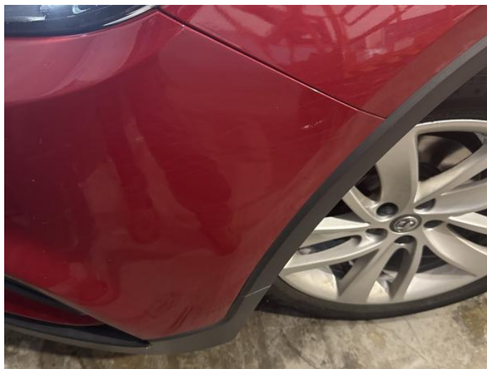
2: Bumper Front Scratched 25 to 100mm Thru Paint
