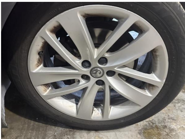
3: Wheel nsf Scratched Over 50mm
