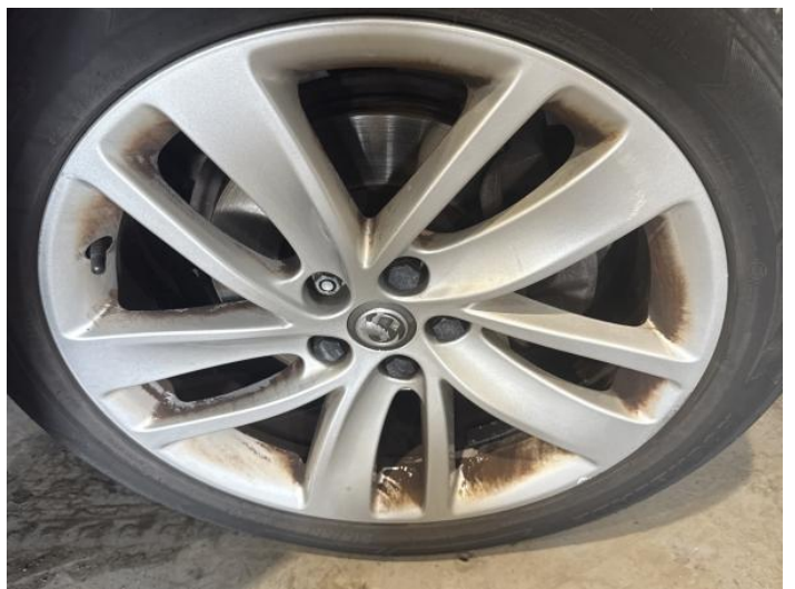
14: Wheel osf Scratched Up To 50mm
