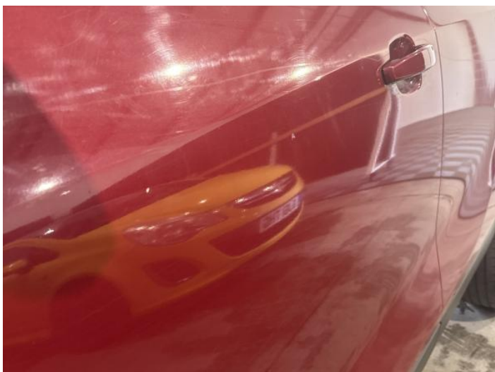
5: Door nsf Scratched Over 25mm Thru Paint
