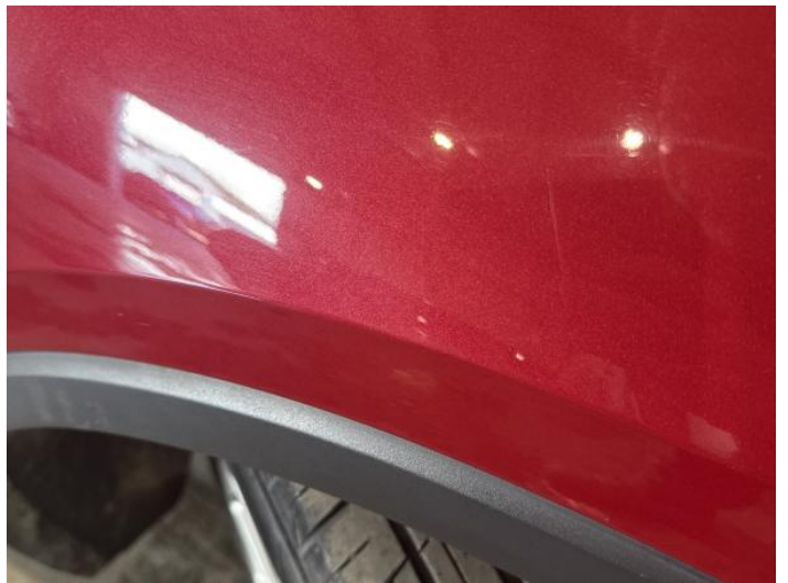
12: Wing osf Scratched UpTo 25mm Thru Paint
