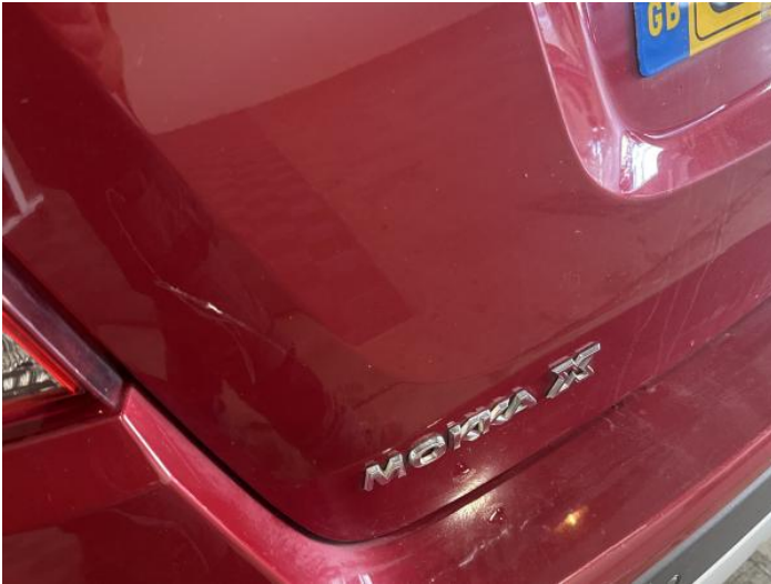
9: Tailgate Scratched Over 25mm Thru Paint
