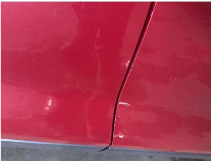
11: Door osr Scratched Over 25mm Thru Paint
