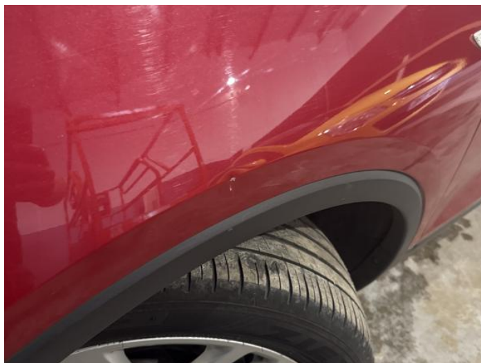
4: Wing nsf Dented With Paint Damage
