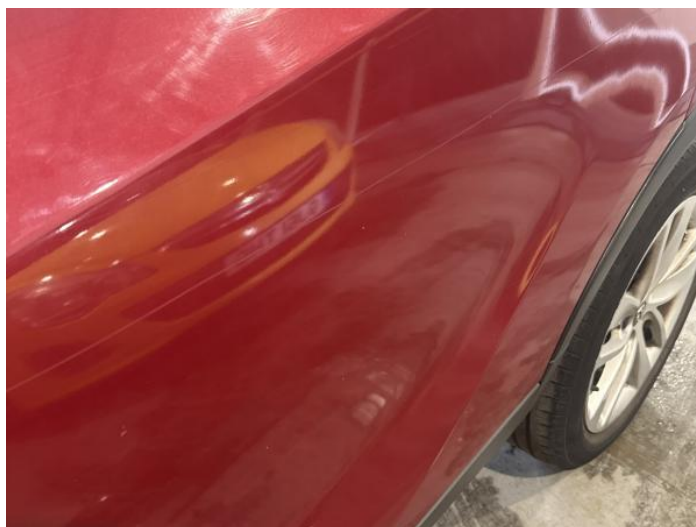
6: Door nsr Scratched Over 25mm Thru Paint
