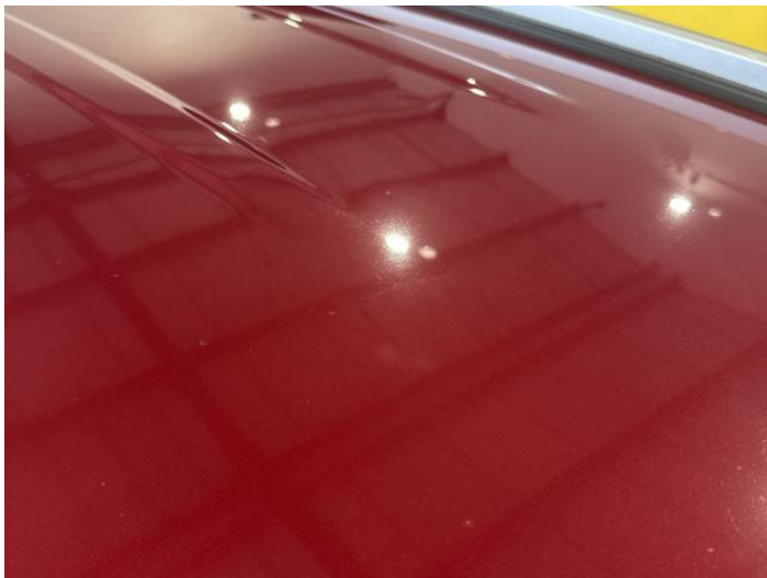
15: Roof Dented Over 30mm
