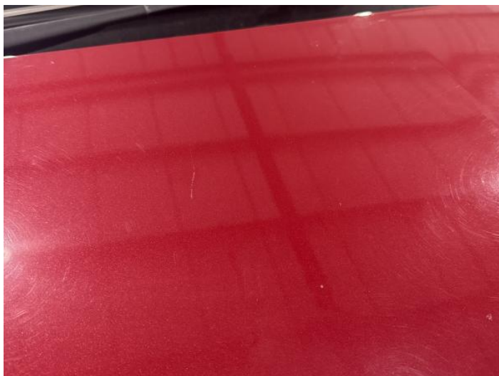
1: Bonnet Scratched Over 25mm Thru Paint
