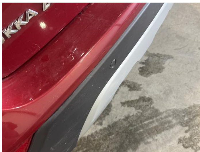
8: Bumper Rear Scratched Over 100mm Thru Paint
