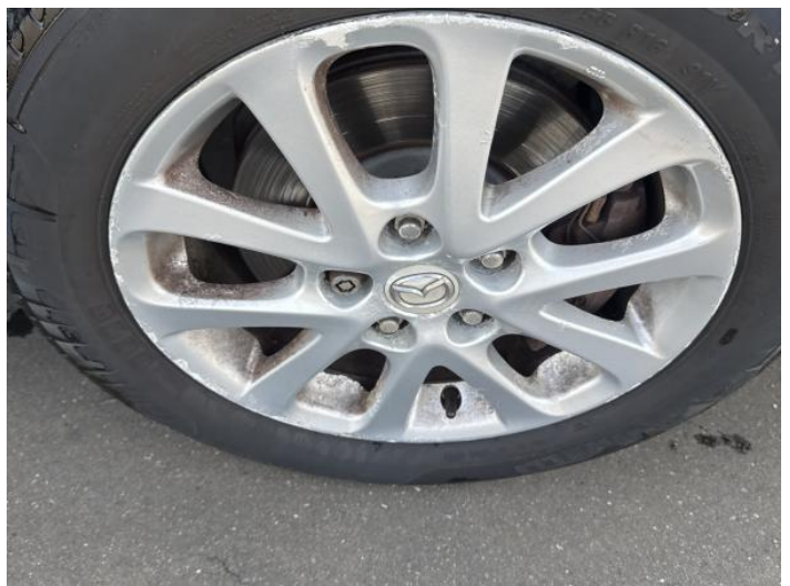
20: Wheel osf Scratched Up To 50mm
