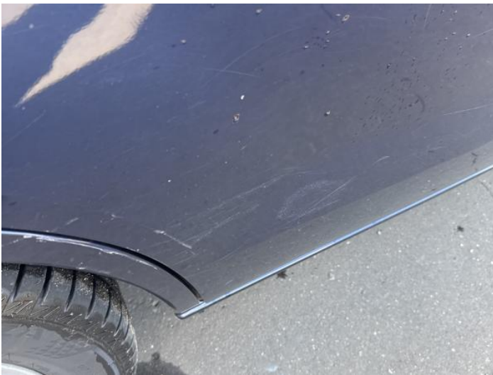
17: Door osr Dented With Paint Damage
