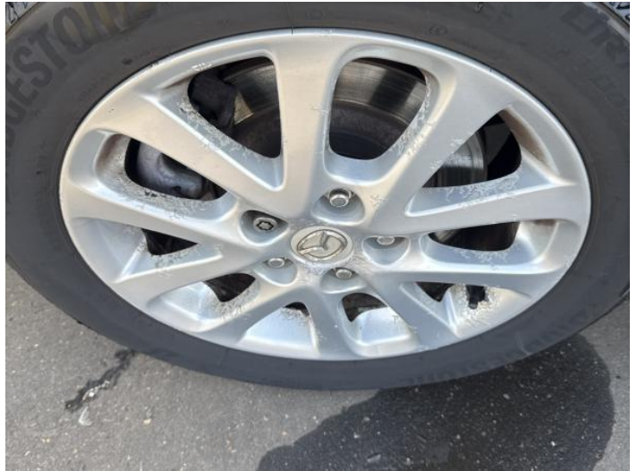
16: Wheel osr Scratched Over 50mm
