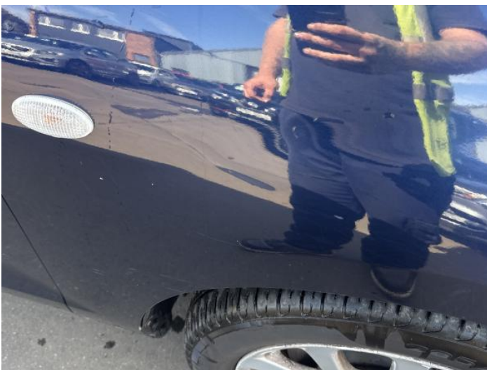
19: Wing osf Scratched Over 25mm Thru Paint
