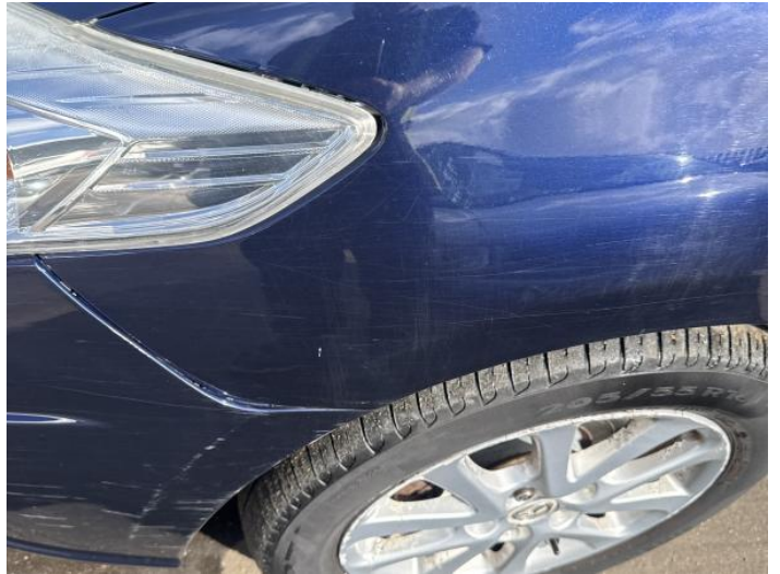
4: Wing nsf Dented With Paint Damage
