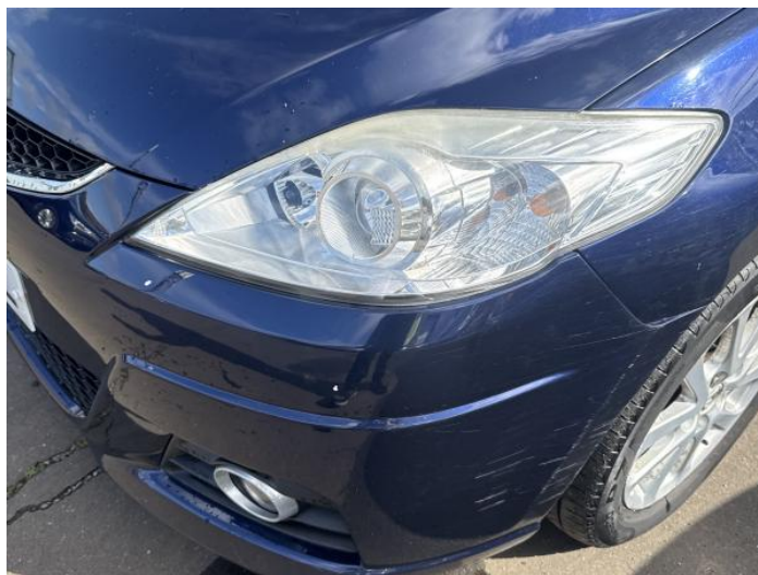
2: Bumper Front Scratched Over 100mm Thru Paint
