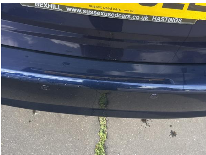
11: Bumper Rear Chipped Multiple Chips
