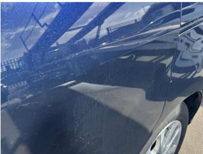
7: Door nsr Dented Between 10mm + 30mm
