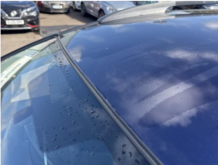
5: Roof Dented Over 30mm
