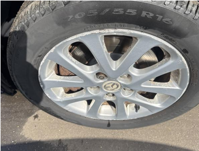
3: Wheel nsf Scratched Over 50mm
