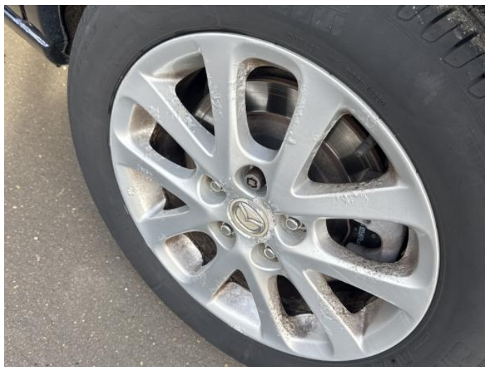
10: Wheel nsr Scratched Over 50mm
