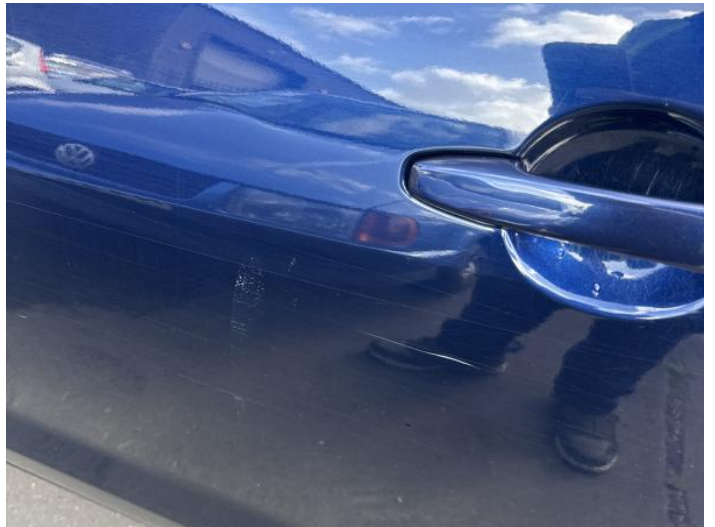
6: Door nsf Dented With Paint Damage
