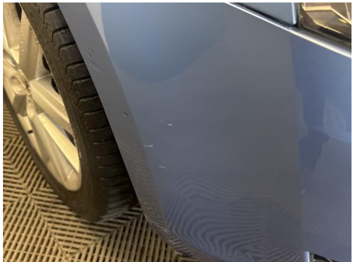
2: Bumper Front Scratched Over 100mm Thru Paint
