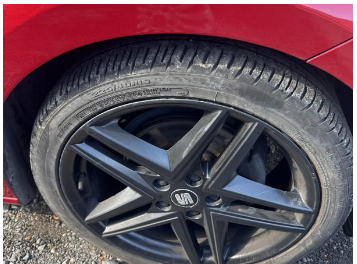
20: Wheel osf Scratched Up To 50mm
