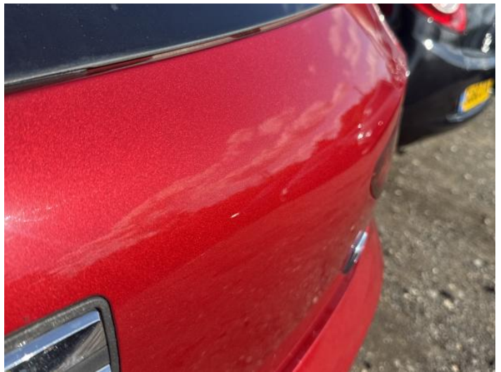
12: Boot Lid Dented Over 2 UpTo 10mm
