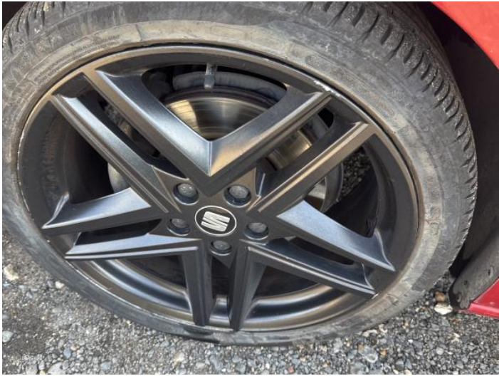
4: Wheel nsf Scratched Over 50mm
