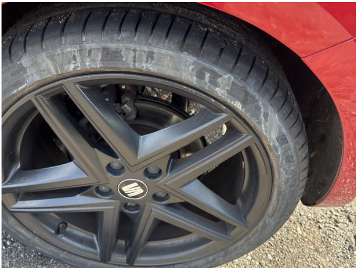
8: Wheel nsr Scratched Up To 50mm
