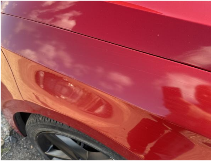
3: Wing nsf Poor Previous Repair Poor Paint
