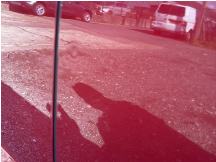
6: Door nsr Dented 2 Or Less UpTo 10mm
