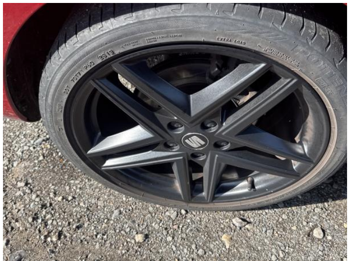
18: Wheel osr Scratched Up To 50mm
