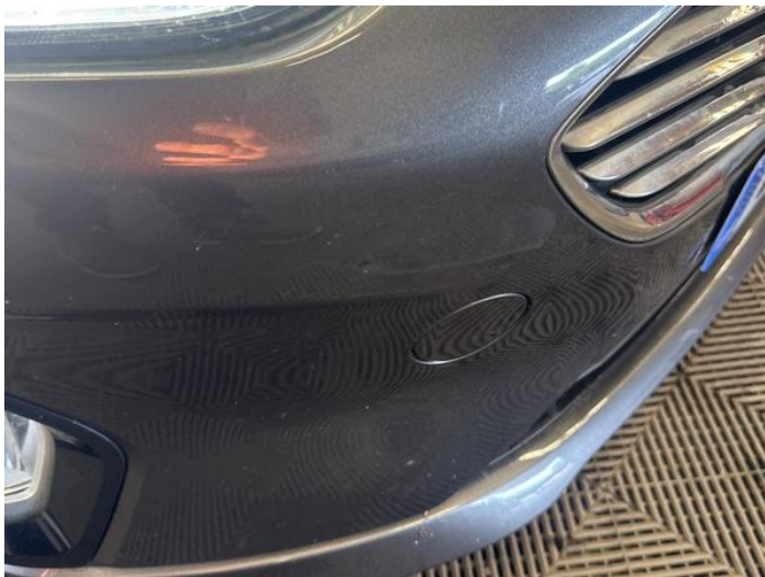
3: Bumper Front Scratched Over 100mm Thru Paint
