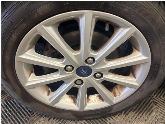
4: Wheel nsf Scratched Over 50mm
