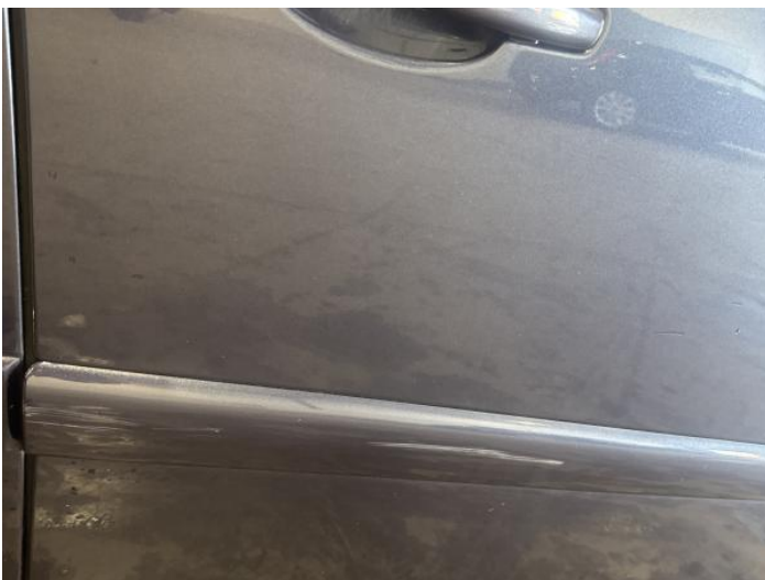
7: Door osf Scratched Over 25mm Thru Paint
