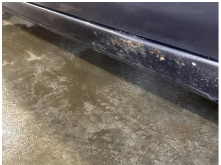
6: Sill os Rusted Over 5mm
