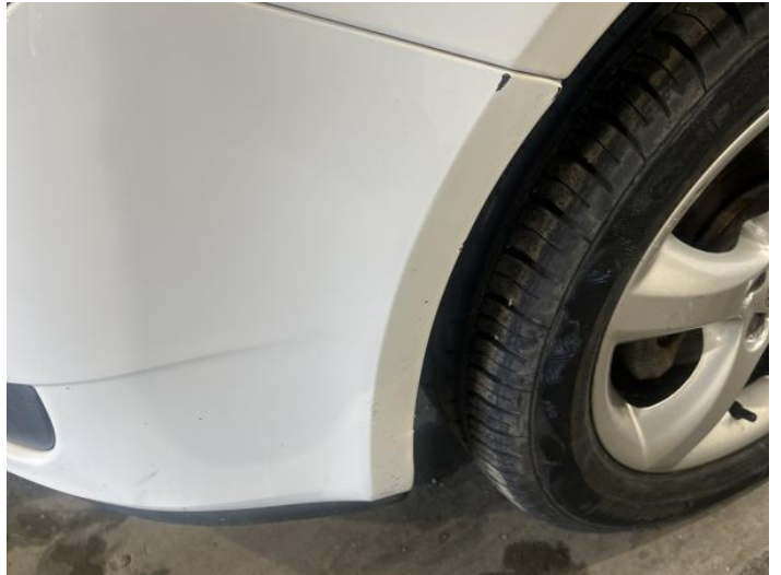
10: Bumper Front Scratched UpTo 25mm Thru Paint
