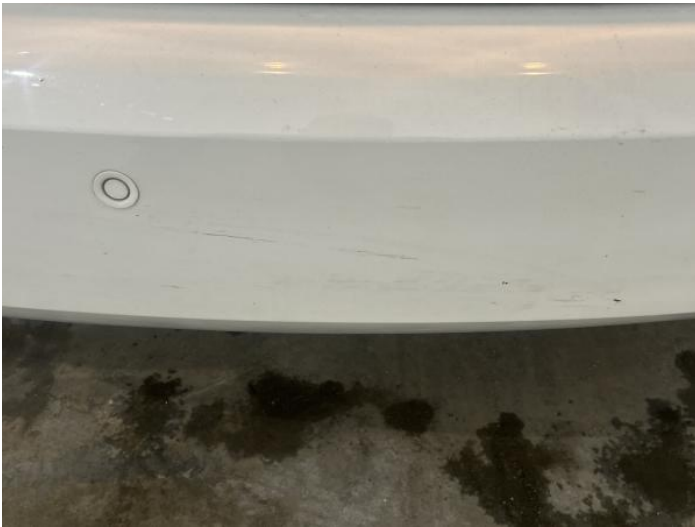
5: Bumper Rear Scratched 25 to 100mm Thru Paint
