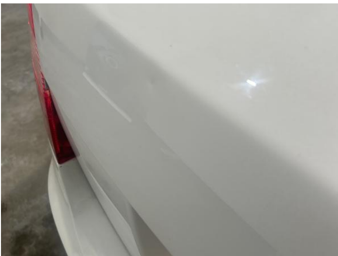
13: Tailgate Dented 2 Or Less UpTo 10mm
