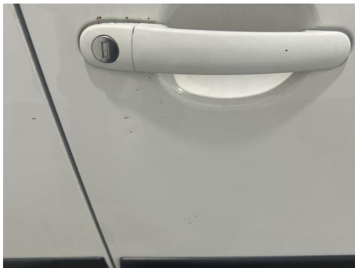
2: Door osf Chipped Multiple Chips
