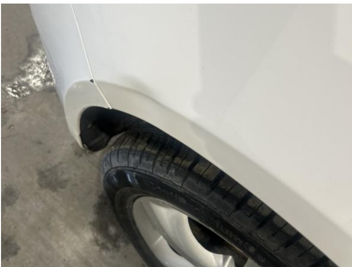
7: Wing nsf Dented Over 30mm
