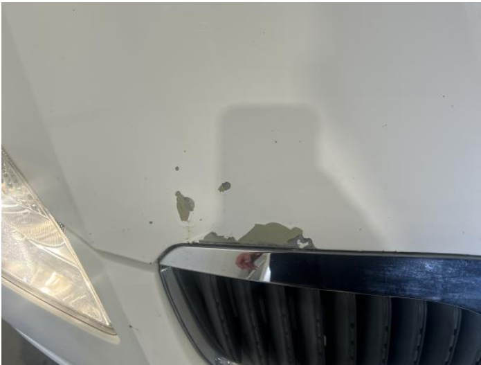
11: Bonnet Poor Previous Repair Paint Flake
