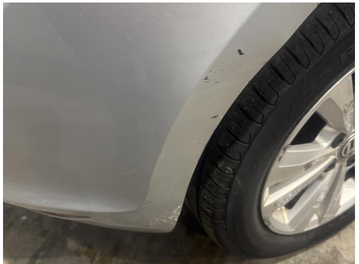
8: Bumper Rear Scratched Over 100mm Thru Paint
