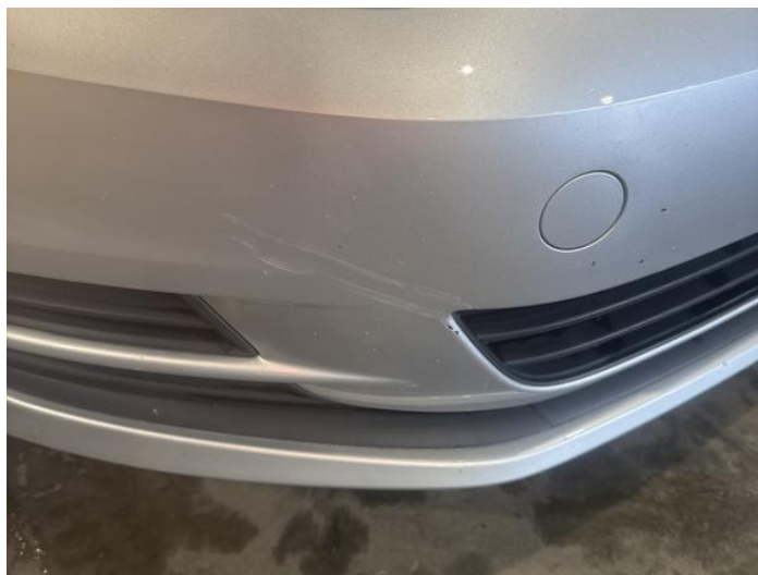
2: Bumper Front Scratched Over 100mm Thru Paint
