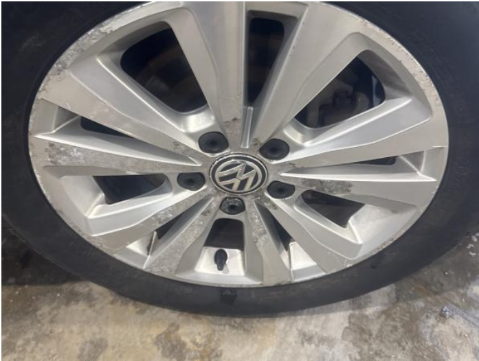
3: Wheel osf Scratched Over 50mm
