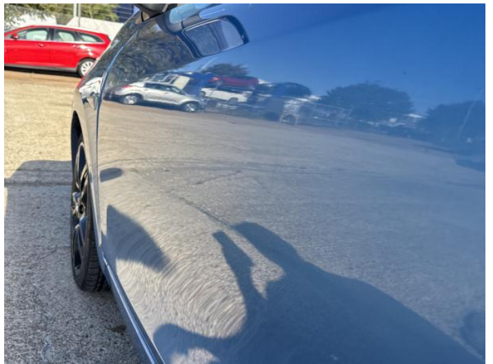
6: Door nsf Dented With Paint Damage
