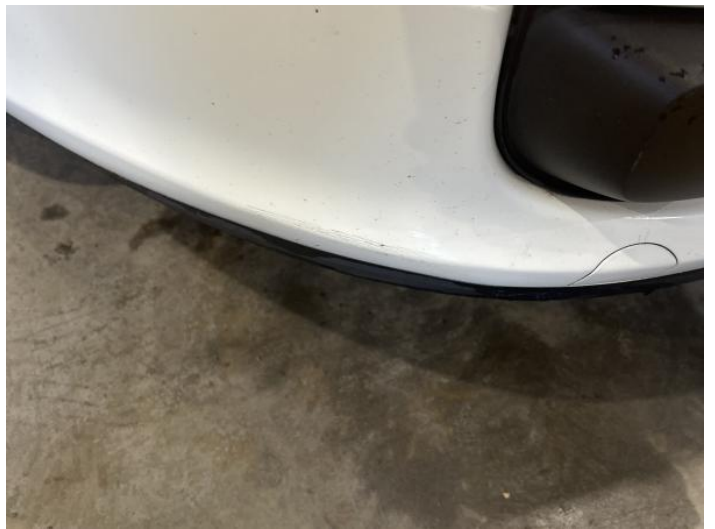
6: Bumper Front Scratched 25 to 100mm Thru Paint
