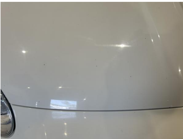
7: Bonnet Chipped Multiple Chips
