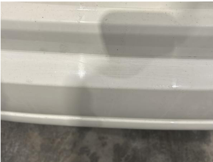
5: Bumper Rear Scratched 25 to 100mm Thru Paint
