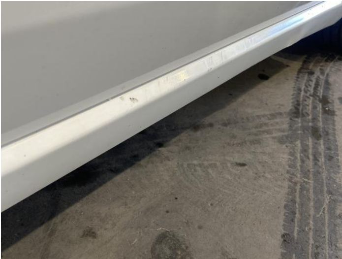
3: Sill os Scratched Over 25mm Not Thru Paint
