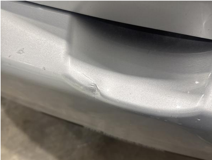
9: Bumper Rear Dented With Paint Damage
