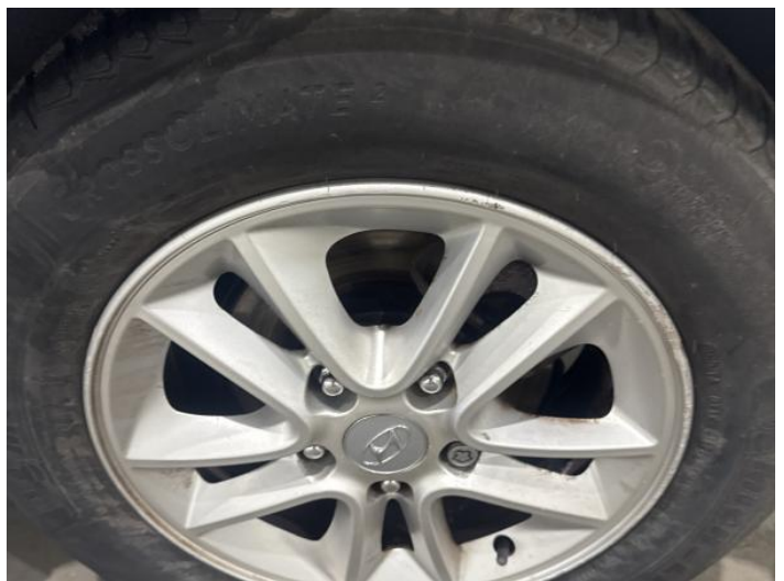
8: Wheel nsr Scratched Over 50mm
