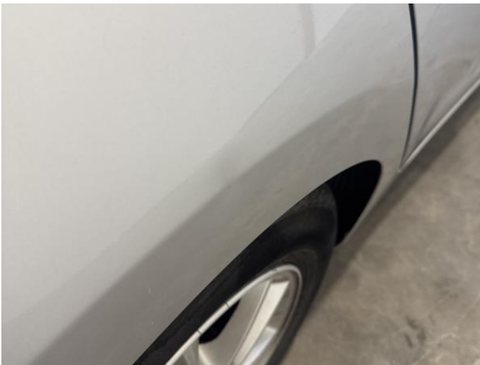
11: Qtr Panel osr Dented Between 10mm + 30mm
