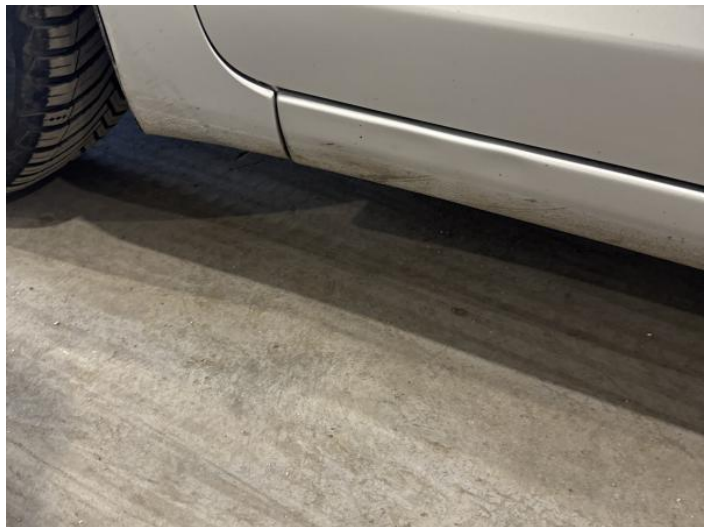
6: Sill ns Dented Over 30mm
