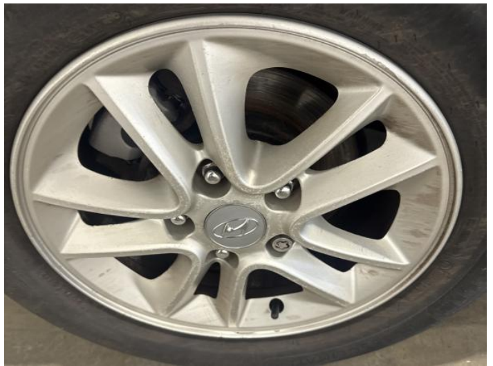
12: Wheel osr Scratched Over 50mm
