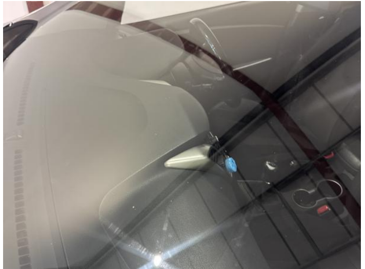
4: Screen Front Chipped UpTo 10mm
