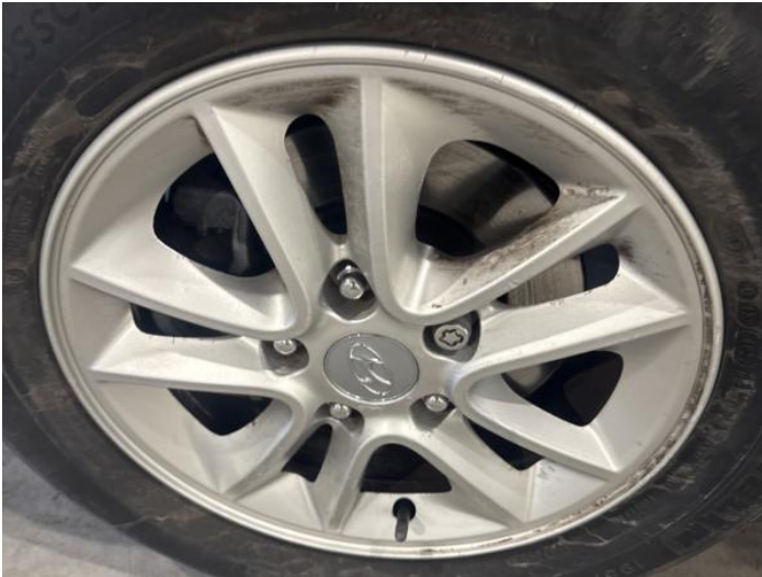
3: Wheel nsf Scratched Up To 50mm
