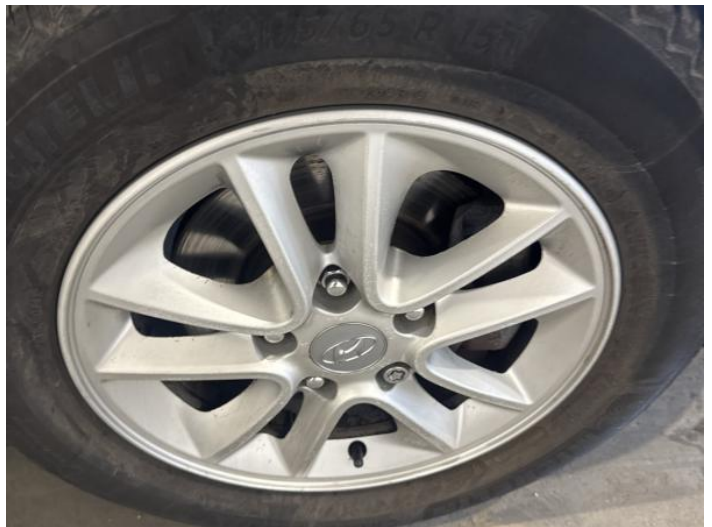
16: Wheel osf Scratched Over 50mm
