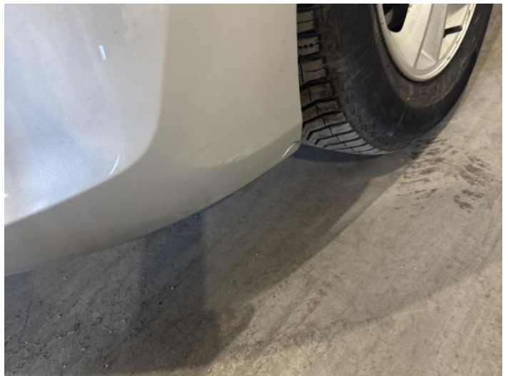
2: Bumper Front Cracked UpTo 25mm
